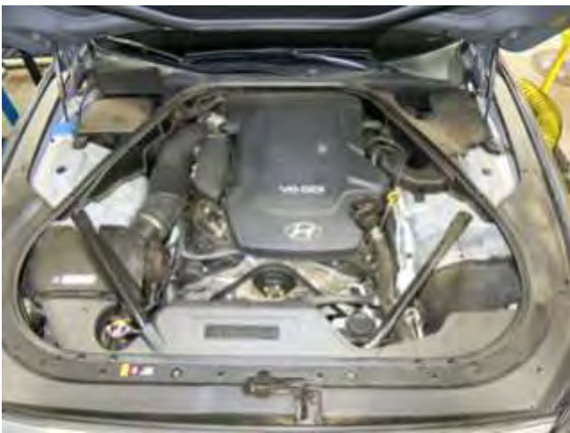
STOCK INTAKE INSTALLED
