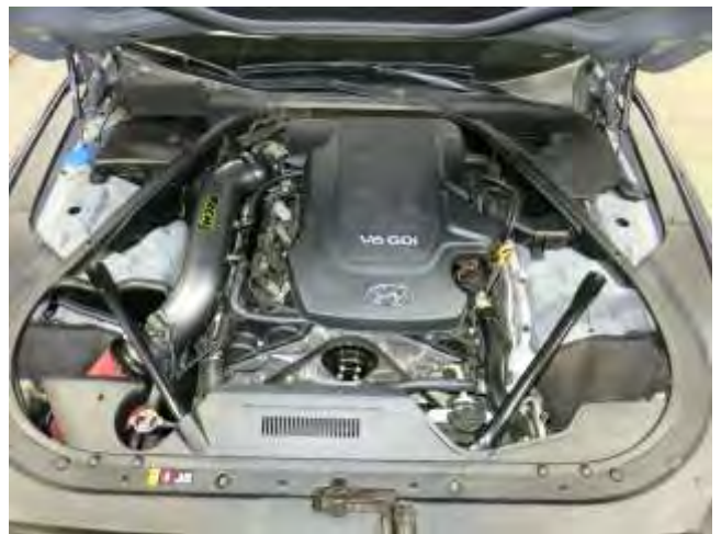
AEM INTAKE INSTALLED
