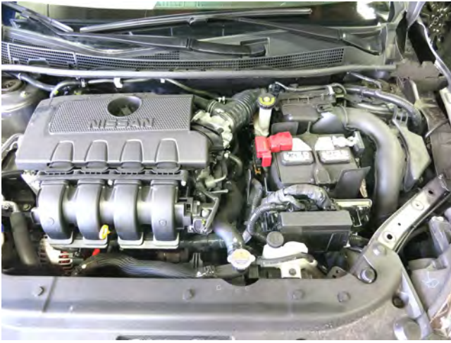
STOCK INTAKE INSTALLED
