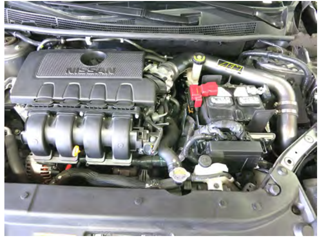
AEM INTAKE INSTALLED
