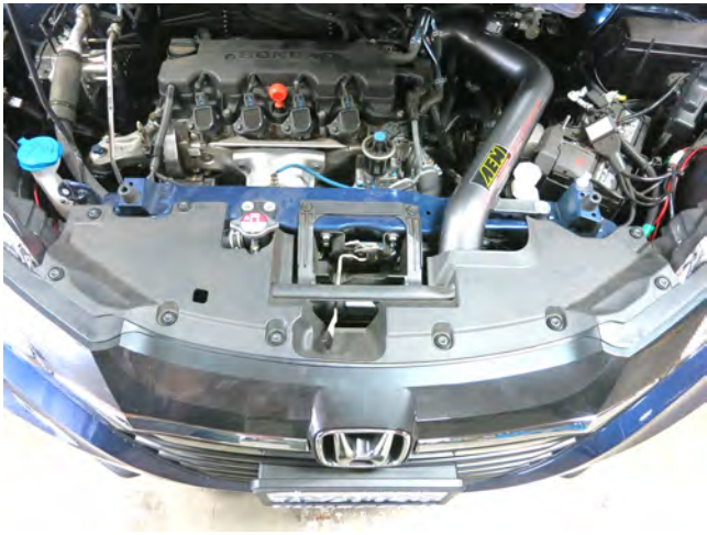
m. Reinstall the plastic radiator shroud you removed in step 2a/b, adjust intake tube for best fitment, then tighten the hose clamp at throttle body coupler and the bolt at intake tube bracket.
