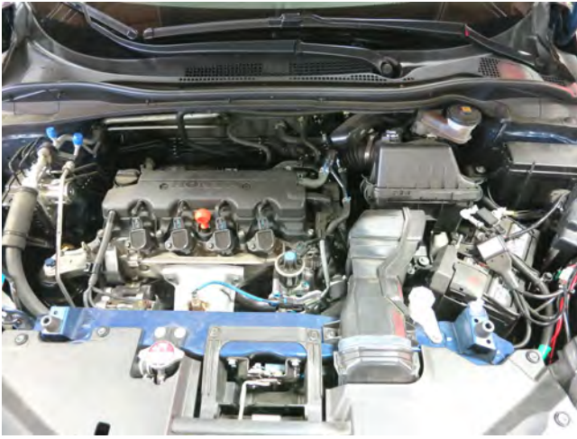
STOCK INTAKE INSTALLED
