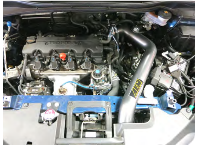
AEM INTAKE INSTALLED
