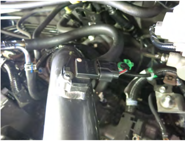
l. Reconnect the MAF sensor harness.
