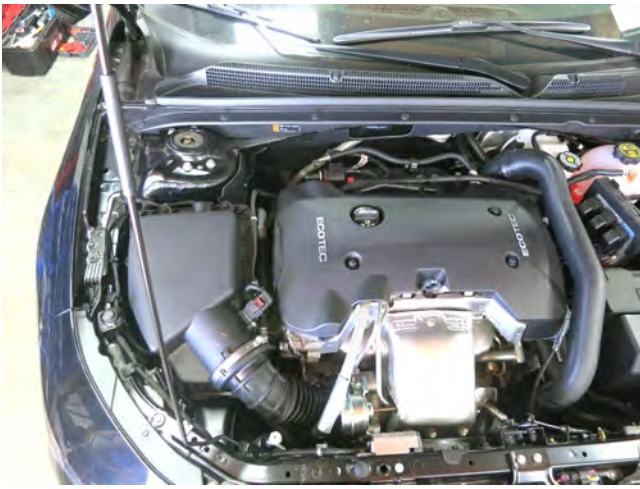
STOCK INTAKE INSTALLED
