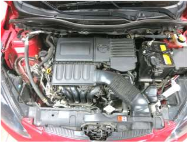
STOCK INTAKE INSTALLED
