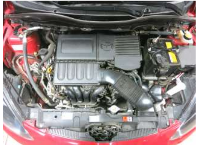
AEM INTAKE INSTALLED
