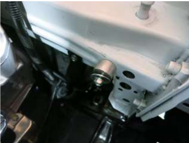
c. Install the supplied aluminum spacer, washer, and bolt onto the threaded hole where the alternator harness bracket was removed in step 2i. Leave the assembly loose.
