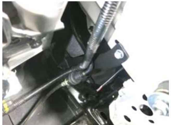
d. Install the supplied clutch hardline relocation bracket using the M6 bolt removed in step 2i. Make sure the alignment tab rests in the cutout on the frame rail.
