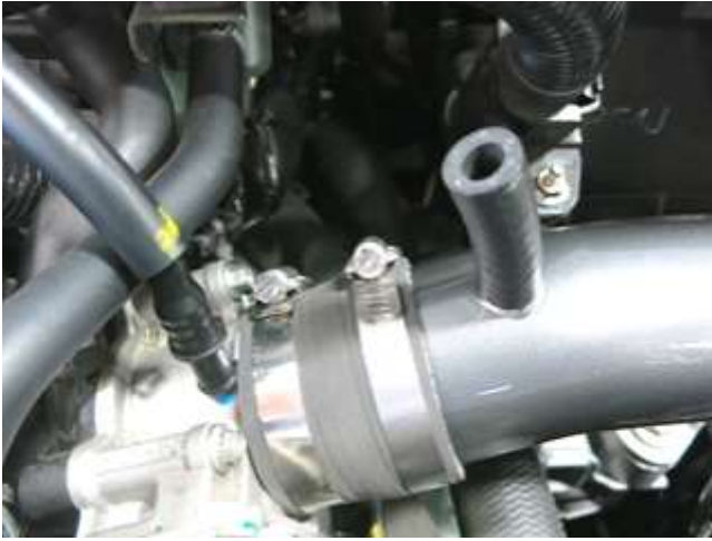
m. Install the supplied 3/8" hose onto the intake tube nipple.
