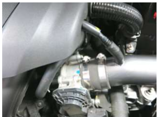
n. Insert the PCV line into the hose. Finally, reinstall the engine cover.
