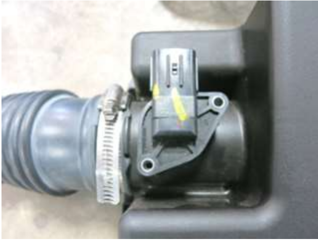
n. Remove the (2) Phillips head screws holding the MAF sensor to the upper air box. Then, remove the MAF sensor. The MAF sensor will be reused with the AEM intake system.
