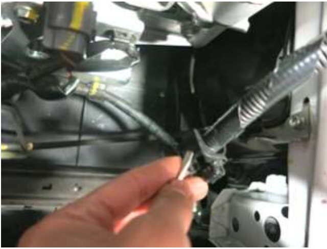
k. Use a small flathead screw driver to release the harness clip from the harness. You will reattach this in step 3e.
