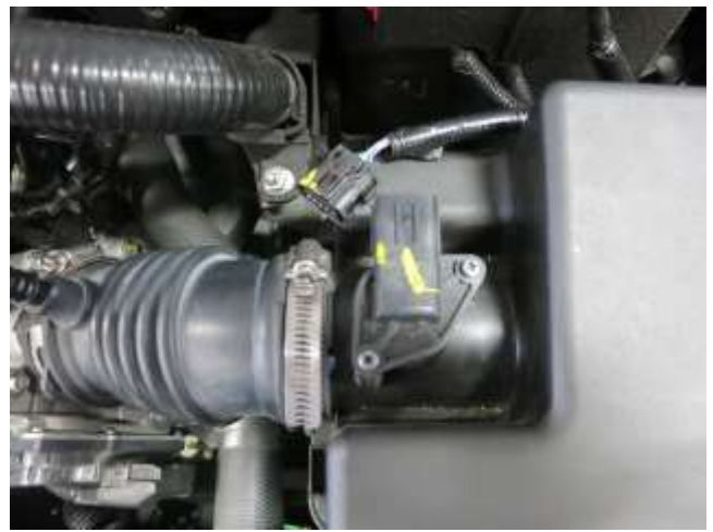
b. Unplug the harness from the MAF (Mass Air Flow) sensor.
