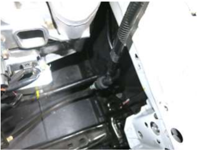
m. Remove the bracket from the clutch hardline grommet. Do not discard any factory components.
