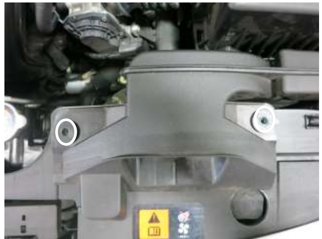
d. Use a 10mm socket and ratchet to remove the (2) M6 bolts holding the intake snorkel to the radiator shroud. Do not discard any factory hardware.
