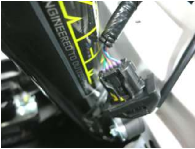
k. Connect the supplied MAF harness extension to the MAF sensor. Then connect the other end to the MAF harness on the vehicle.
