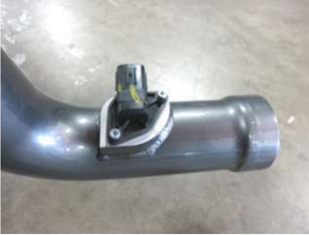
a. Install the MAF sensor to the AEM intake tube with the (2) supplied M4 bolts.
