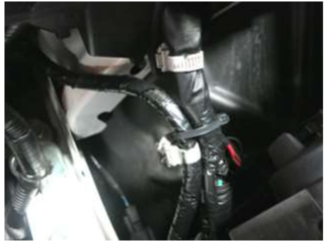
l. Use the supplied zip tie to tie the MAF sensor harness to the main fuse box harness.
