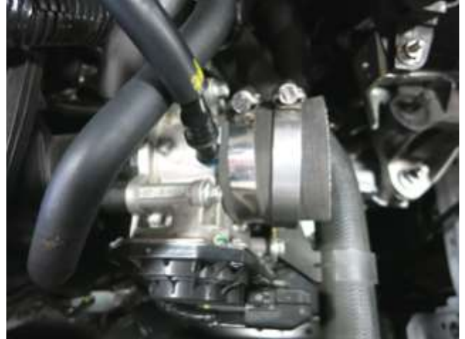
b. Install the tapered coupler onto the throttle body, making sure the smaller end goes onto the throttle body. Use the supplied #36 hose clamp to tighten the coupler onto the throttle body to 30 in-lbs.
