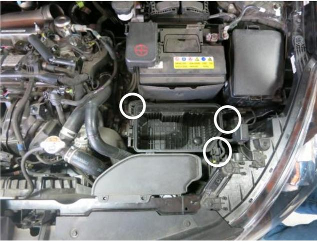
g. Remove the (3) bolts that secure the lower air box housing with a 10mm socket and ratchet.
