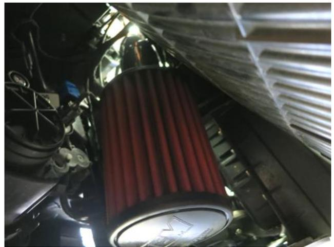
j. Install the filter onto the AEM intake tube, then tighten the band clamp with a 8mm nut driver.
