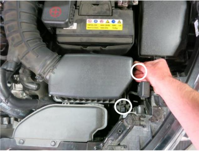
e. Detach the 2 latches from the air box lid from the lower air box housing and remove airbox lid and intake hose.
