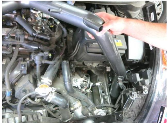
d. Pull the filter end up and over the frame rail to its proper place.
