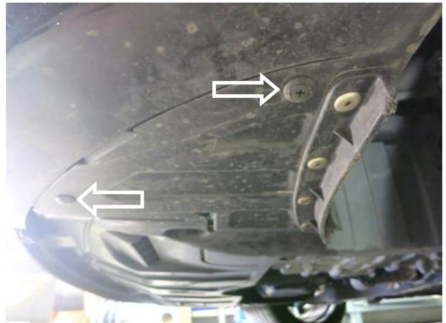
h. Remove the 2 fender liner clips by using a #2 phillips screwdriver.
