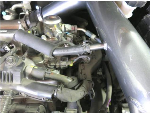
m. Reinstall the PCV hose to the AEM intake tube using the stock spring clamp.
