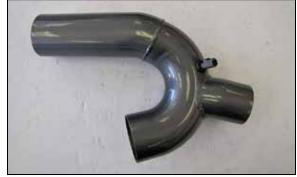
16. Install the provided grommet and inlet air temperature sensor into the AEM® intake tube as show.
