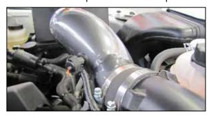
18. Reconnect the inlet air temperature sensor electrical connection.
