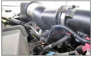
2. Disconnect the inlet air temperature sensor electrical connect and remove the tape around the harness connector.
