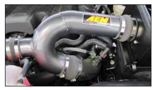
17. Install the AEM® intake tube into the couplers at the turbo inlet tubes and then into the coupler at the filter adapter, adjust the tubes for best fit and then secure with the provided hose clamps.
