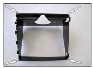
7. Install the small edge trim onto the bottom of the heat shield as shown using the provided super glue to secure it in place.
