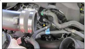
14. Install the provided coupler hose (5-302) onto the passenger side turbo inlet hose and secure with the provided hose clamp.
