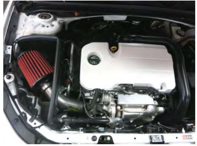
AEM INTAKE INSTALLED
