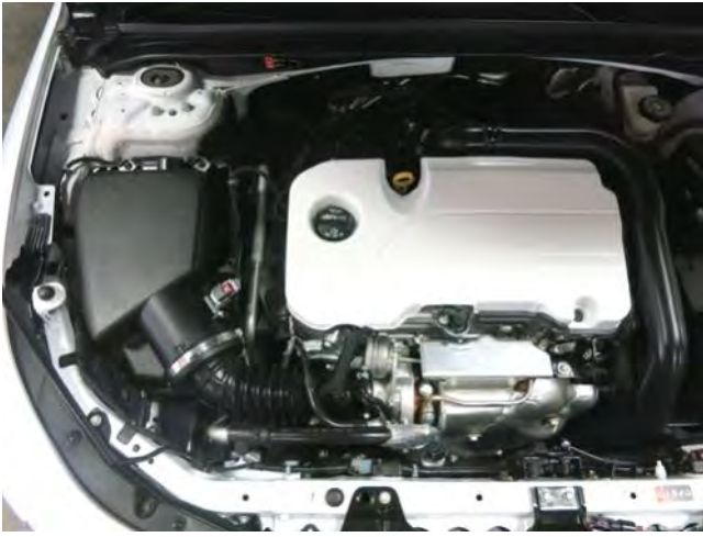
STOCK INTAKE INSTALLED
