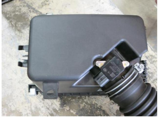
h. Remove the MAF sensor from the air box using a screwdriver. The MAF sensor will be reinstalled in step 3b. **Note: handle the MAF sensor with care.**
