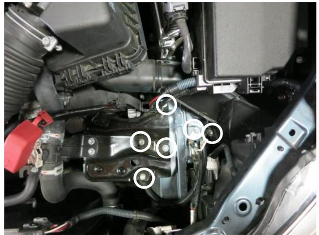
d. Remove the 4 bolts that hold the battery tray, the bolt for the ground cable to chassis, and the one bolt for the air box scoop. BOLTS WILL BE REUSED IN STEP 3d.
