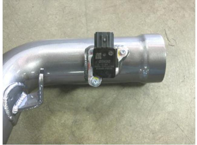
b. Install the MAF sensor onto the AEM intake tube with the supplied M4 fasteners.
