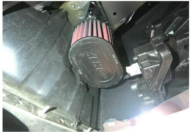
h. Install the air filter onto the tube. Be sure to have clearance around the filter before tightening the clamp.
