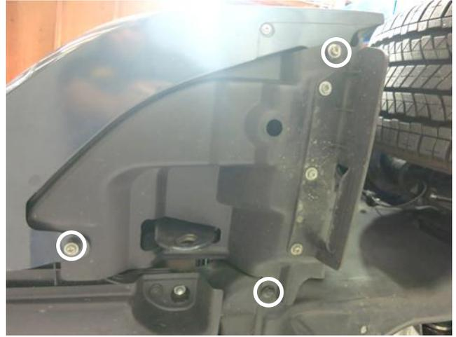
f. Lift the vehicle up with a floor jack and secure it with jack stands. Remove the 2 bolts and the push clip on the fender liner as shown. Then pull back fender liner for access.
