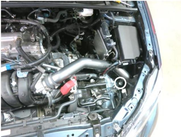
c. Tighten the rubber mount to the air box mounting hole, then install the AEM intake tube. **DO NOT TIGHTEN THE NUT UNTIL INSTRUCTED TO DO SO IN THE LATER STEP.**
