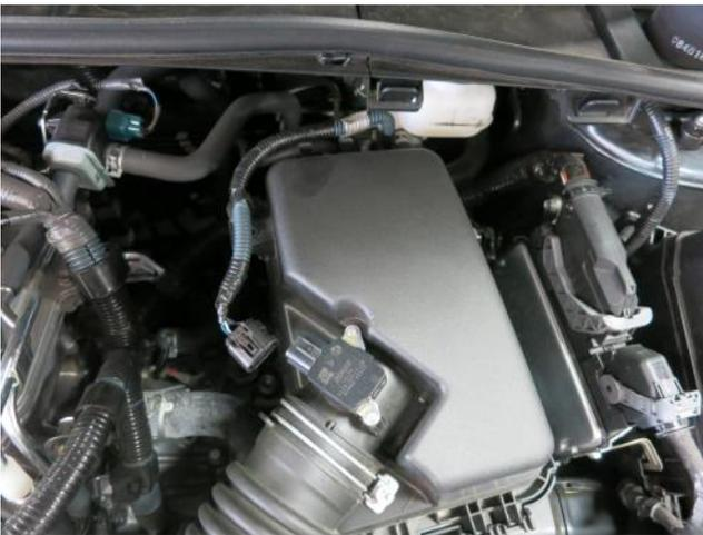
c. Unplug the Mass Air Flow sensor electrical connector.
