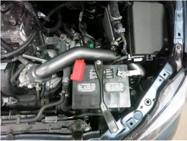
e. Secure the battery by tightening the bolt on the core support, then tighten the nut on the battery strap.
