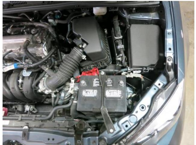
b. Disconnect both battery terminals, remove bolt that holds battery strap, then remove battery from vehicle.
