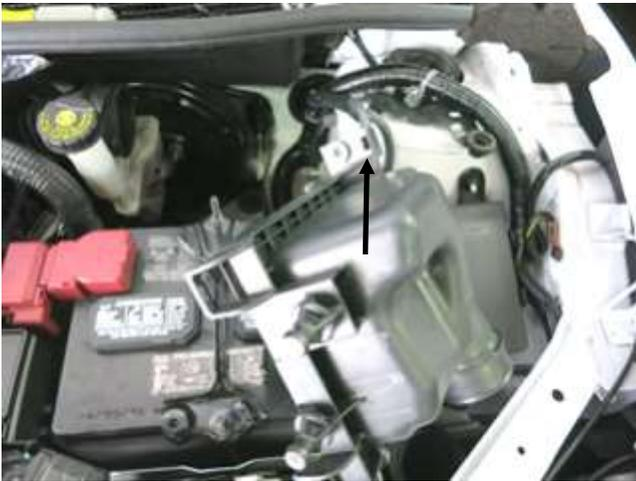
g. Pull up on the air box to release it from its grommets, disconnect the coupler, and turn the box on its side as shown to access the next wire tie. Release the harness from the air box and remove the air box from the engine bay.
