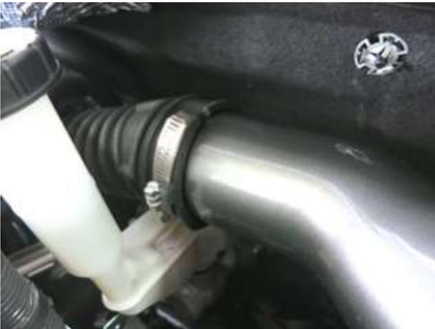
c. Connect the upper intake tube to the factory coupler. Soapy water can be used to help installation. Tighten this hose clamp at this time.
