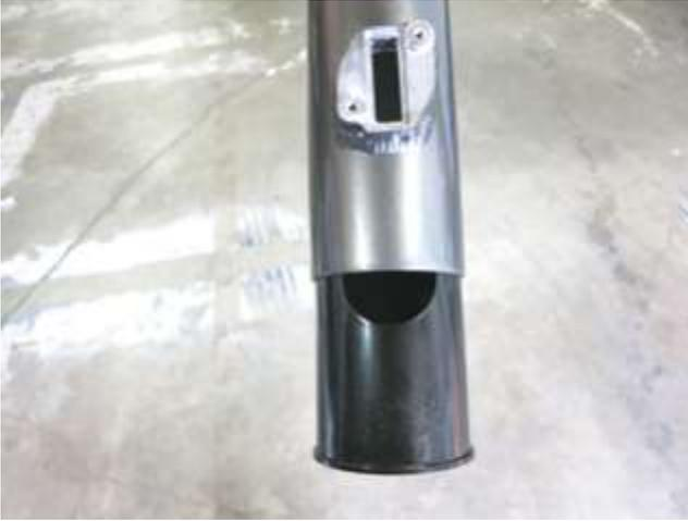
a. Align the hole in the venturi insert with the MAF pad as show and fully insert into the lower intake tube. **Note: The venturi insert is necessary for proper engine function and performance.**
