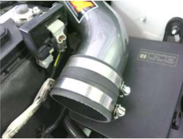
e. Install the provided coupler and hose clamps on to the upper intake tube. Position the coupler so it overlaps the upper intake tube about 1 inch and tighten the upper hose clamp.
