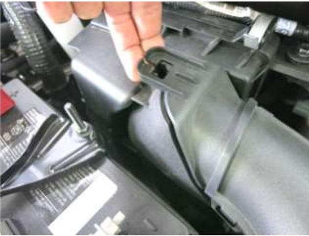
a. Lift up the plastic tab on the air box resonator so it is unclipped.
