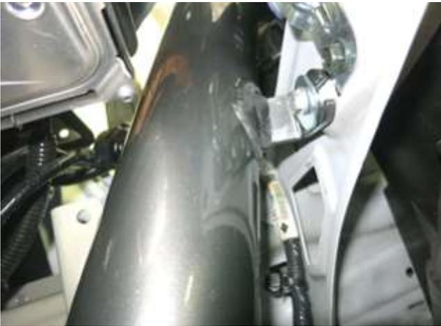
g. Loosely secure the lower intake tube to the inner fender using the bolt and washer provided.
