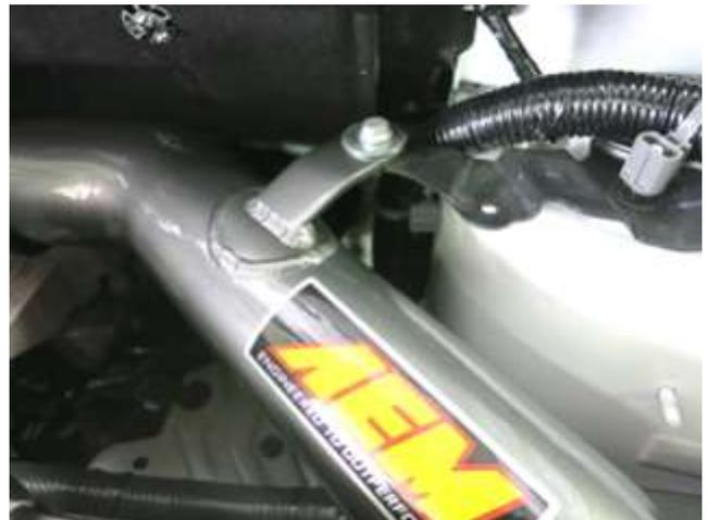
d. Loosely secure the upper intake tube to the factory metal bracket using the provided bolt and washer.
