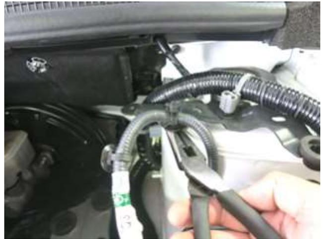
h. Release the final wire tie from the metal bracket as show and move the MAF harness down and out of the way.
