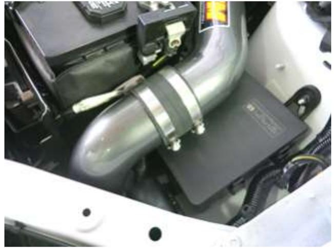
f. Bring the lower intake tube into the engine bay from under the fender well area and insert it into the coupler. Use care not to scratch the finish on your new intake tube. Masking tape can be used on the sharp edge of the core support if necessary. Do not fully tighten the lower hose clamp at this time.
