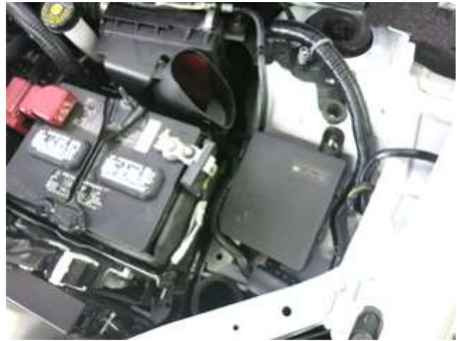
b. Lift the resonator duct up and out of the engine bay. Pull gently to release it from the grommet.
