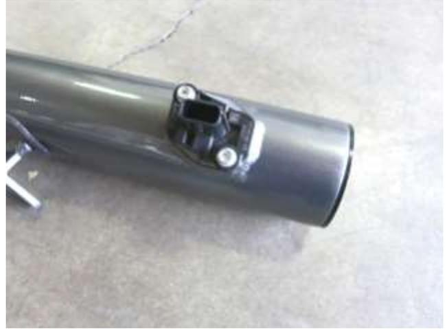
b. Install the MAF sensor into the lower intake tube using the screws removed in step 2p.
