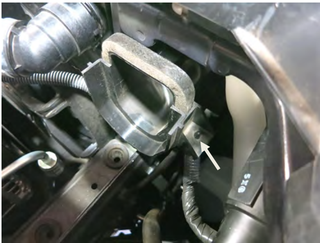
m. Release the wiring harness from the passenger side air ducting.
