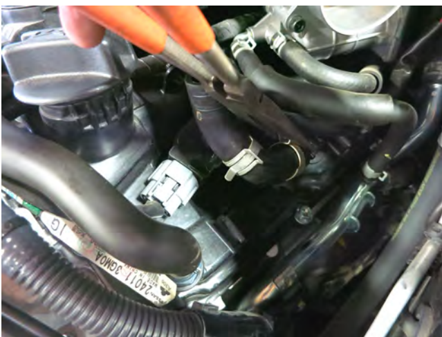
i. Remove the driver side PCV hose and set aside. This will be reused.
