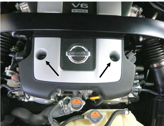
a. Remove the front half of the engine cover by loosening its two bolts.
