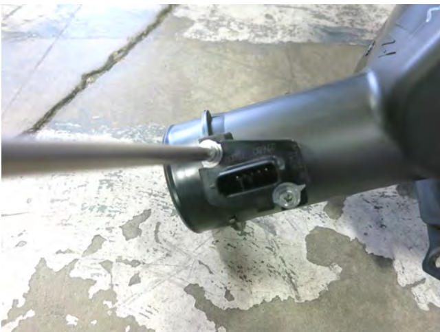
o. Remove both MAF sensors from their factory air boxes. Note: Do not discard any of your stock equipment.
