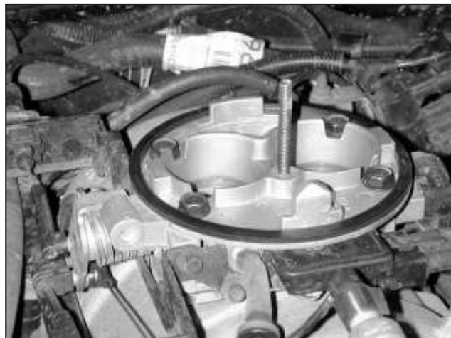
i. Remove stock inner plenum support. Place gasket on throttle body and install stud as shown.
