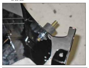
b. Install the supplied rubber mount onto the heat shield using an M8 washer and nut.
