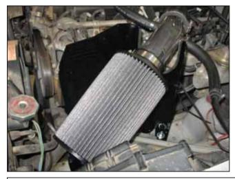
k. Install the AEM® Dryflow™ air filter onto the end of the pipe. Push the air filter over the intake pipe until the stop in the air filter is reached. Use a #48 clamp to secure the air filter onto the intake pipe.
