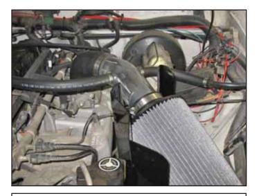
AEM® intake system installed
