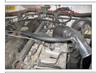
i. Install the hose between the valve cover breather nipple and the breather nipple on the engine side of the intake pipe. Secure using two of the supplied 1" hose clamps. Trim hose to fit.
