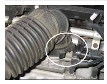
d. Loosen the hose clamp on the throttle body. This is done by simply pulling outward on the plastic hose clamp grips.
