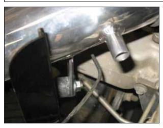
h. Slide the intake pipe into the elbow until the mounting bracket aligns with the rubber mount on the heat shield. Secure the pipe to the bubber mount using the remaining M8 washer and nut.
