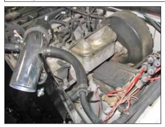
j. Install the supplied breather hose between the hard plastic charcoal canister hose and the nipple on the driver side of the intake pipe. Secure using the remaining 1" hose clamps. Trim hose to fit.
