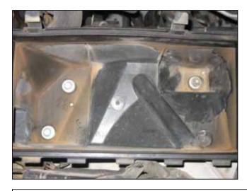
f. Remove the air filter from the housing. Remove the two bolts and the one nut from inside the filter housing. Lift up and remove the air filter housing base.
