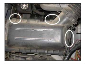
e. Unclip the three clamps securing the air filter housing lid to the base. Remove the lid and the inlet hose.
