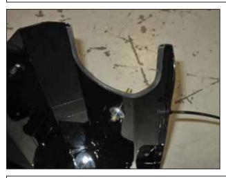
d. Install the rubber edge trim onto the top edge of the heat shield where the pipe passes through.
