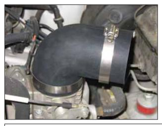
g. Install the 90 degree coupler onto the throttle body and secure using the supplied #48 hose clamps.
