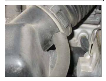
c. Remove the rubber hose connecting the hard plastic charcoal canister hose to the air filter housing.
