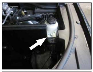
g. Place the power steering reservoir tab ove the AEM heatshield bracket and install the factory M8 bolt. Do no tighten completly at this time.
