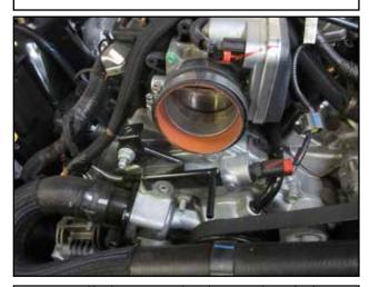
p. Install the supplied coupler (N) on the throttle body along with the supplied hose clamps (O).
