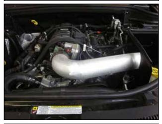
t. With the AEM air intake tube properly aligned, tighten all hose clamps, nuts and bolts installed in previous steps.
