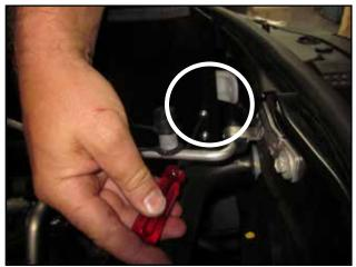
h. Attach the heat shield to the bracket installed in step 3-e) with supplied M6 bolts (L).
