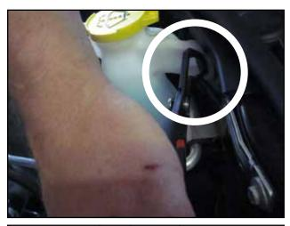
Remove the plastic clip securing the windshield washer fluid reservoir to the core support.
