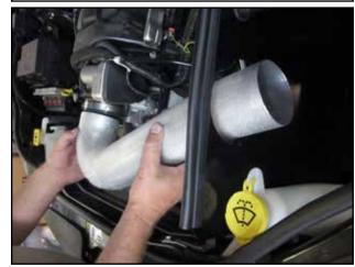
q. Install the AEM air intake tube (A)
