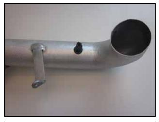
m. Insert the IAT sensor into the AEM air intake tube as shown.
