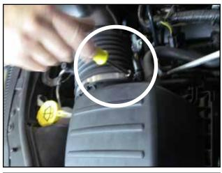
f. Loosen the hose clamp at the air box.
