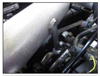
This is how the bracket should look when properly installed.
