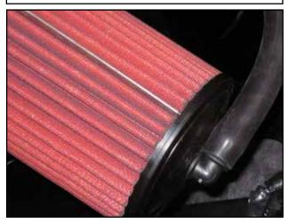
Intall the elbow vent fitting (E) to the AEM air filter (D) top and attach the supplied 5/8" id hose (F) to the fitting.
