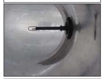
n. This is what the IAT sensor probe looks like inside the tube when sensor is properly inserted.
