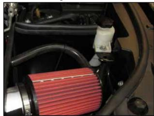
w. Wrap the zip tie (I) around the vent hose to hold it in place. And snap the tree into the hole.
