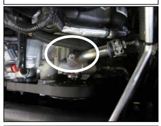
Loosen and remove the M8 bolt from the power steering pump housing. This bolt will not be reused.
