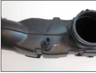
From the factory air inlet tube, twist and remove the IAT sensor.
