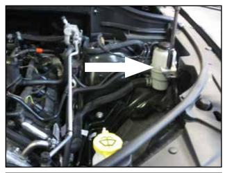
k. Loosen and remove the M8 bolt securing the power steering fluid resvervoir. The bolt will be reused later.
