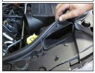
Detach the air inlet duct from the rubber edge trim.
