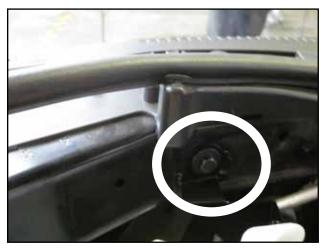
e. Install the supplied heat shield bracket (B) to the core support with the factory 6 mm bolt. Do not completely tighten the bolt at this time.
