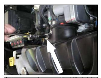
d. Loosen and remove the M6 air inlet chamber mounting bolt.
