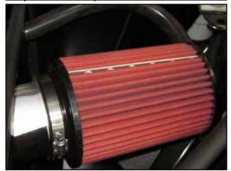
v. Attach the filter to the AEM air intake tube and attach the vent hose to the vent fitting on the heat shield.
