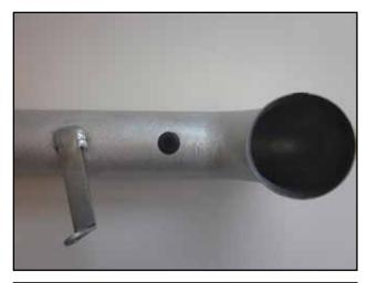
Install the supplied grommet (m) into the hole on the AEM intake tube.
