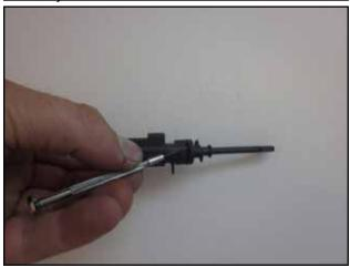
k. Once the IAT sensor is removed, use a suitable tool or pick to remove the small o-ring from the IAT sensor.
