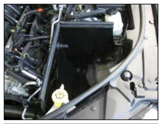
f. Line up the grommets to the two studs and place the heat shield in place; install the thick rubber edge (j) trim on top of the heat shield.
