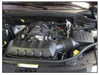
Remove the engine cover by pulling straight up.
