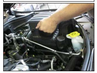
Lift and remove the air box from the engine bay.
