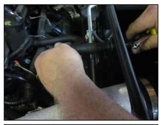
x. Attach the valve cover breather hose to the other end of the straight vent fitting.
