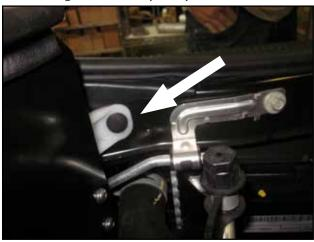
Place the windshield washer reservoir back in its place and reinstall the plastic clip removed from step 2-I).
