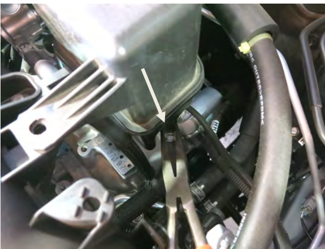
c. Disconnect the PCV hose from the intake resonator by releasing the pressure on the spring clamp.
