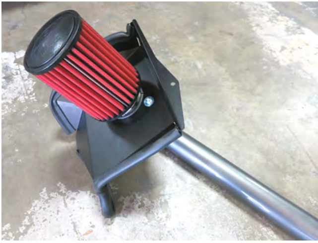
f. Install the AEM DryFlow filter using the provided hose clamp onto the intake tube.
