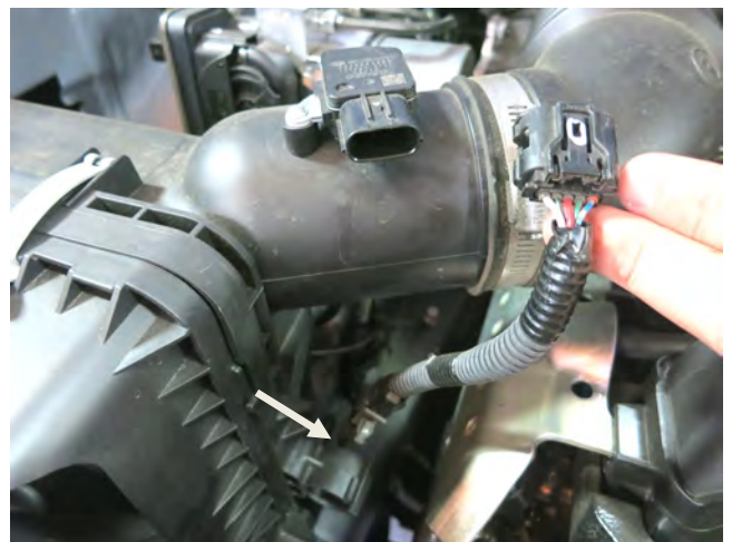
d. Disconnect the Mass Air Flow (MAF) sensor harness from the MAF sensor and the air box.
