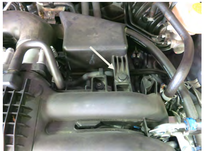
b. Remove the push-in plastic fastener securing the intake resonator to the intake manifold.
