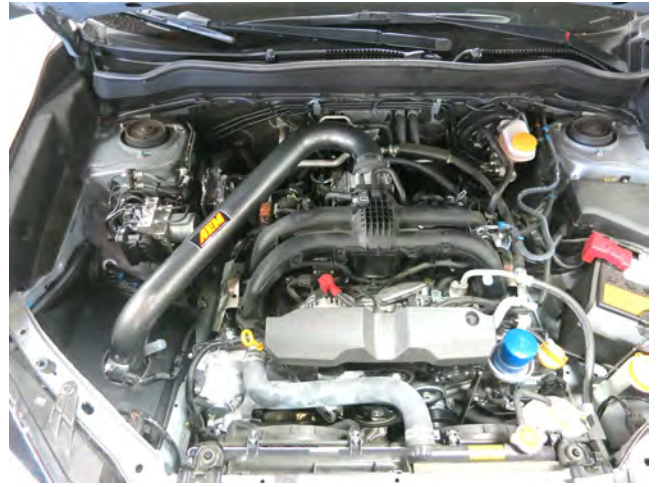
AEM INTAKE INSTALLED
