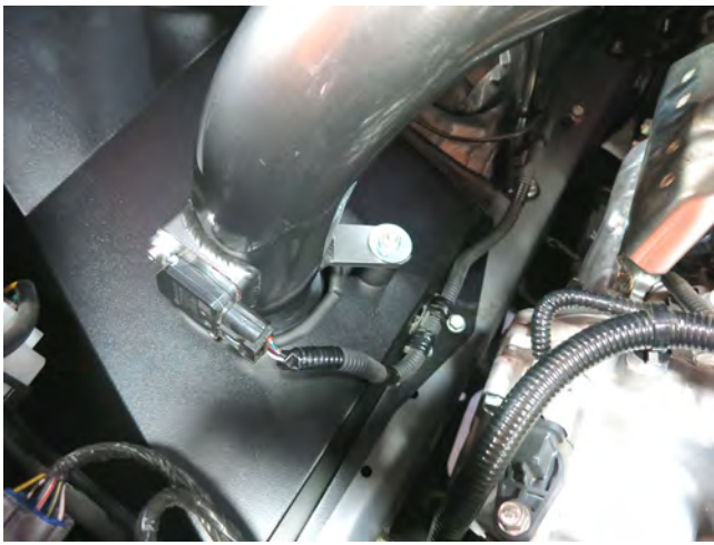
j. Connect the MAF sensor harness to the MAF sensor and secure the harness on the heatshield. Tighten the nut on the bracket to secure the tube.
