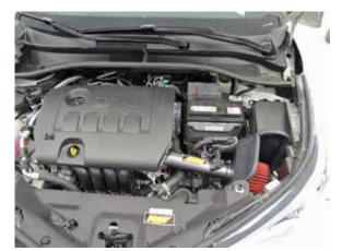
22. Reinstall the core support cover and secure with the factory hardware. Reconnect the negative battery cable.
