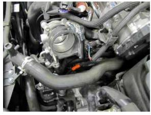
12. Install the provided coupler (08284) onto the throttle body and secure with the provided hose clamp.
