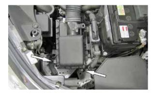
5. Release the two clips that secure the upper air filter housing, then remove the upper housing with the intake tube and crank case breather hose. Remove the factory air filter.
