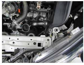
13. Install the fresh air intake tube into the coupler at the heat shield but do not completely tighten the hose clamp at this time to allow some adjustment.
