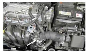
4. Loosen the hose clamp that secures the intake tube to the throttle body. Release the spring clamp that secures the crank case vent hose to the valve cover port and then disconnect the crank case vent hose.
