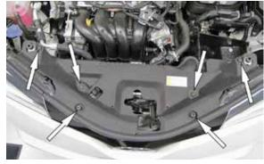
6. Remove the four plastic retaining clips and two hood stops and then remove the core support cover.
