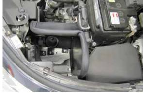
11. Install coupler (08284) onto the heat shield and secure with the provided hose clamp. Set the heat shield assembly onto the inner fender and secure with the hardware provided.
