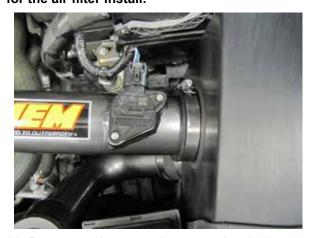
20. Reconnect the mass air sensor electrica connection.
