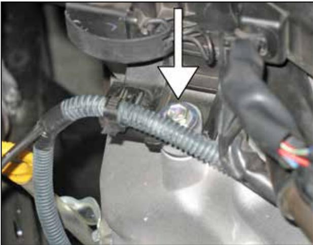
g. Remove the bolt securing the factory air box to the valve cover. Retain this bolt, it will be reused in a later step. Remove the zip ties securing the wire harness to the air box.
