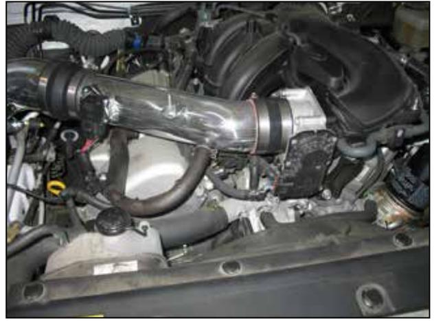
o. Install the PCV hose on the upper intake pipe on the nipple located near the front of the vehicle. Use the factory hose clamp to secure.
