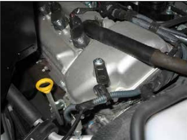
f. Attach the supplied bracket with an M6 bolt and washer.
