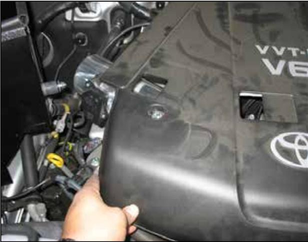
j. Align the bolt installed in step 3b. with the engine cover. Once aligned, remove the engine cover again.
