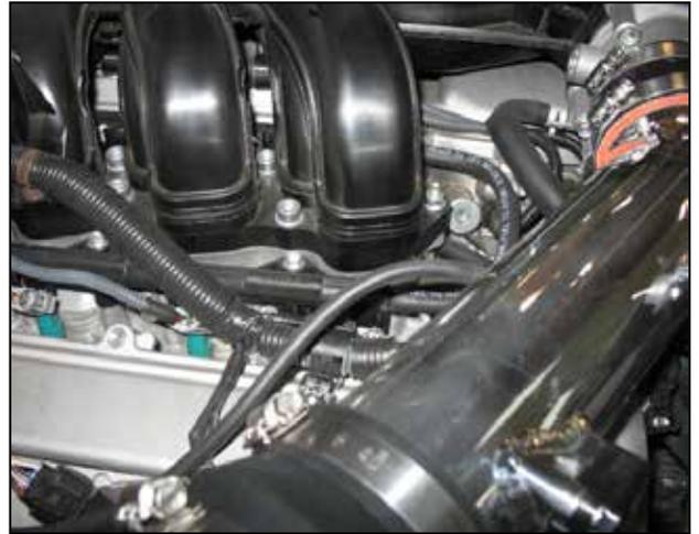
m. Attach the open end of the 5/32 ID hose onto the intake pipe's nipple.
