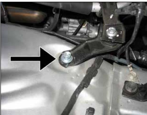
i. Remove the bolt securing the bracket for the A/C line. Retain this bolt as it will be reused in a later step.
