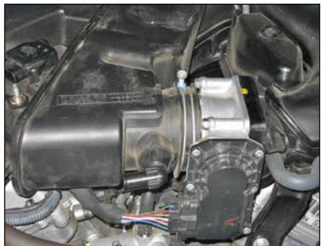
j. Loosen the hose clamp securing the factory air box to the throttle body.
