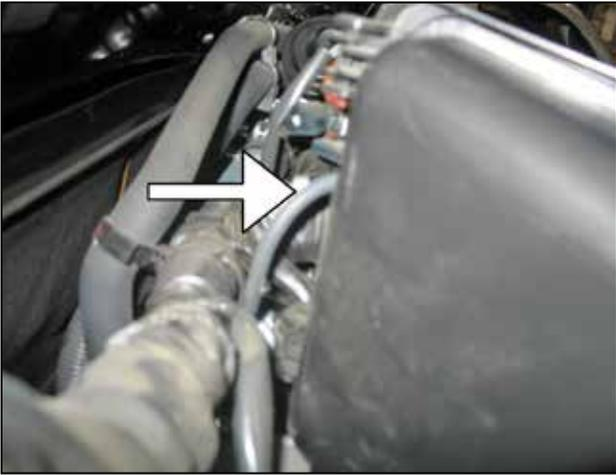
e. Disconnect the breather hose located in the back of the factory intake system; it is the hose connected to the fuel pressure regulator.
