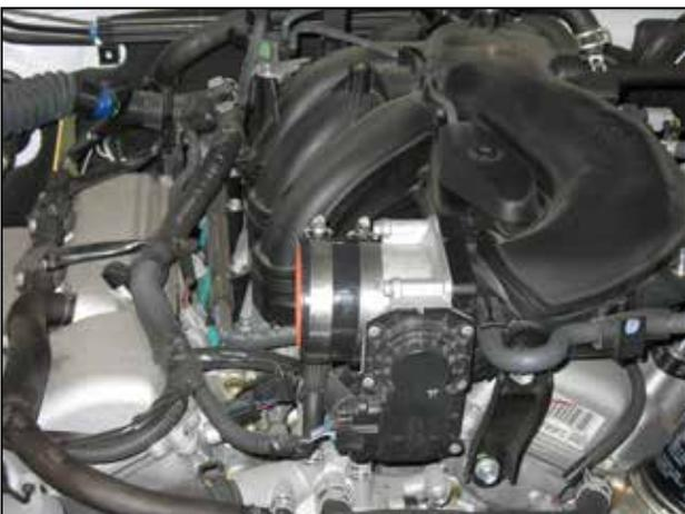
h. Install the silicone coupler to the throttle body using the supplied #48 hose clamp.
