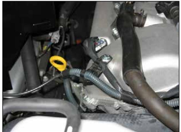
g. Attach the factory zip ties to the bracket installed in step 3f.
