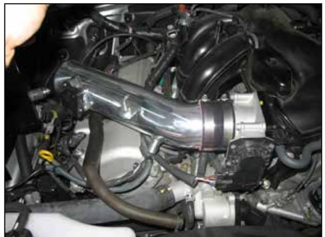
i. Insert the upper intake pipe into the silicone coupler and loosely secure using the another #48 hose clamp.
