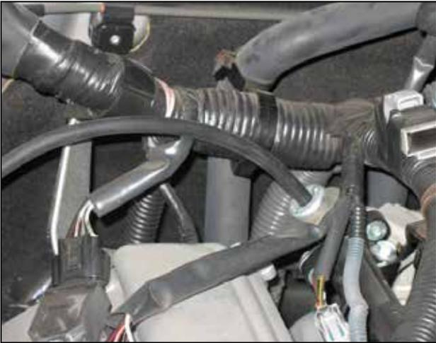
l. Install the 5/32 ID hose onto the fuel pressure regulator.
