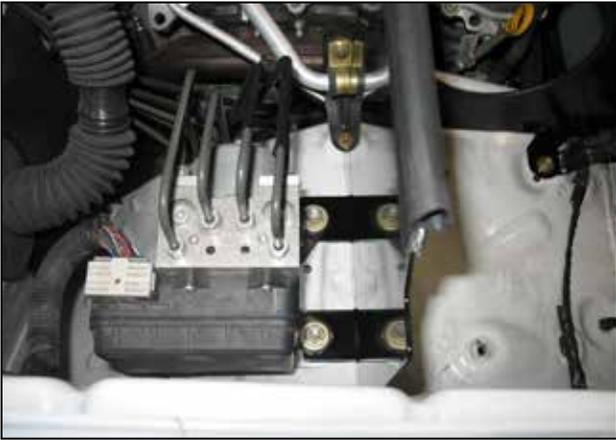
d. Loosen the two nuts securing the ABS module. Tilt the ABS module slightly and slide the heat shield under the ABS bracket.
