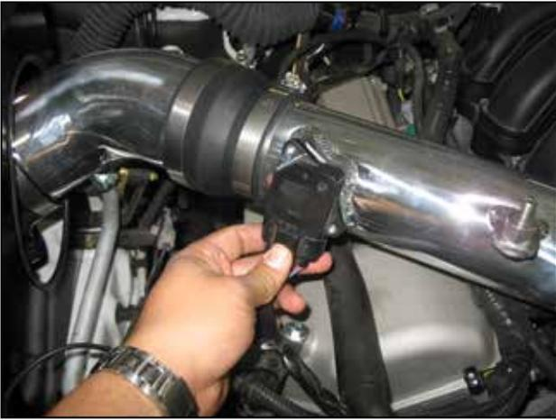
n. Plug the MAF sensor wiring harness into the MAF sensor.
