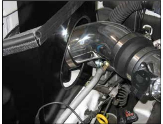
k. Install the screened hose adapter onto the end of the intake pipe. Insert the short intake pipe into the hose adapter and align the pipe's bracket with the rubber mount. Loosely secure the hose adapter and short intake pipe with the provided #56 & #48 hose clamps.
