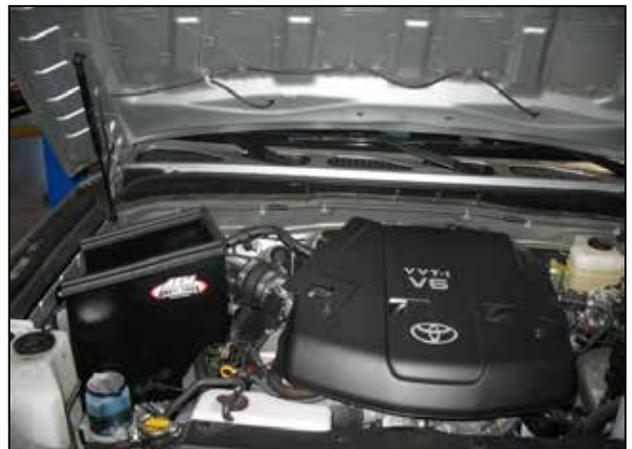
AEM® intake system installed
