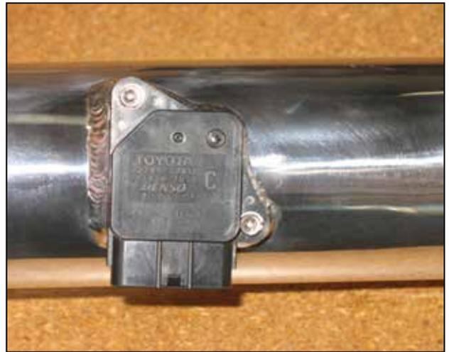
c. Install the MAF sensor in the upper intake pipe using the supplied bolts.
