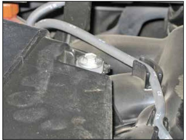
f. Remove the bolt securing the factory intake system to the intake manifold.
