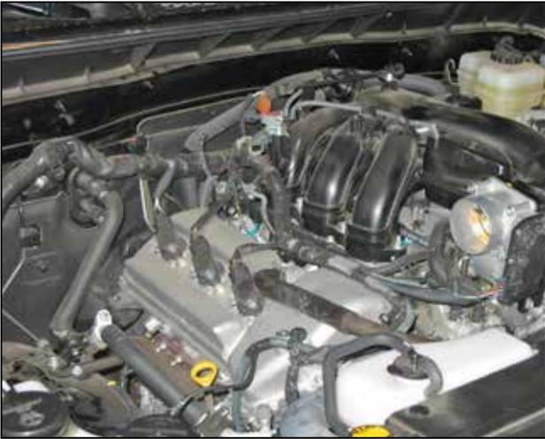
k. Factory air box system removed from the vehicle.
