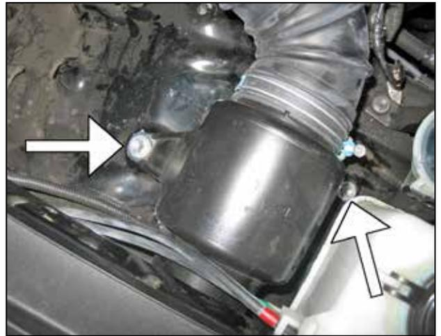
h. Remove the two bolts that secure the intake tube to the fender well. The bolt closest to the front of the vehicle will be reused in a later step.
