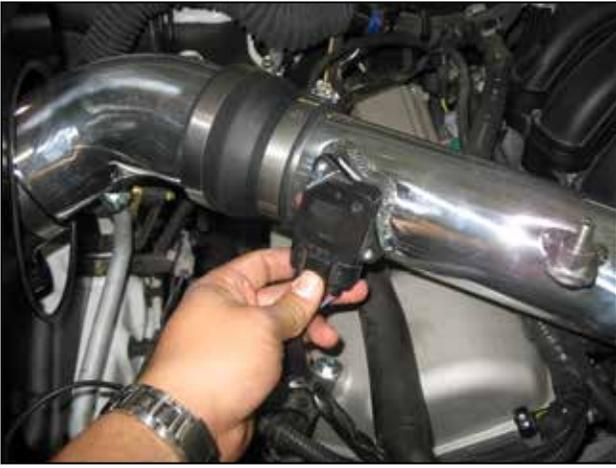
n. Plug the MAF sensor wiring harness into the MAF sensor.
