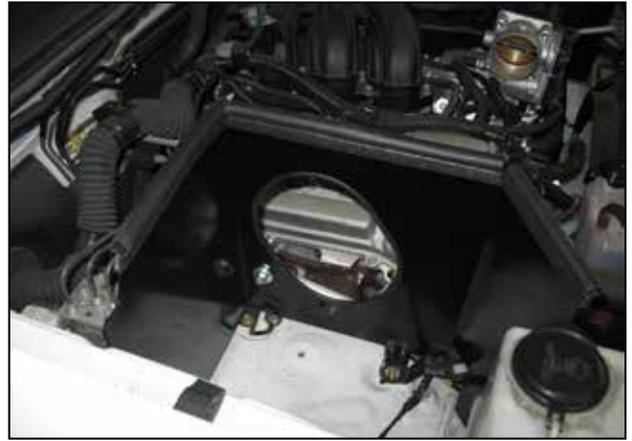
e. Align the heat shield mounting holes with the bolt holes that were exposed during steps 2h and 2i when the bolts were removed. Use the factory bolts to secure the heat shield in place. Install the edge trim, and the rubber edge trim onto the heat shield. Install the supplied rubber mount onto the heat shield using the provided hardware.
