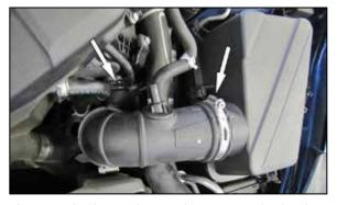
5. Loosen the hose clamps that secure the intake tube to the air filter housing and turbo inlet and then remove the intake tube from the vehicle.
