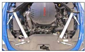
2. Remove the four bolts shown that secure the two strut tower braces to the vehicle and then remove the braces from the vehicle.
