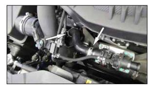
7. Release the spring clamps that secure the passenger side BOV hose to the BOV and intake tube, then remove the Passenger side BOV hose. **NOTE: This hose will be reused.**
