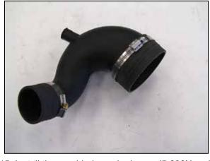
15. Install the provided coupler hoses (5-222N and 08761) onto the Passenger side intake tube (9-0461) and secure with the provided hose clamps.
