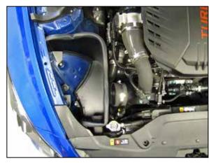
17. Install the passenger side heat shield and secure with the provided hardware.
