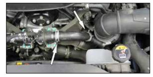
4. Release the spring clamps that secure the driver side BOV hose to the BOV and intake tube, then remove the driver side BOV hose.
