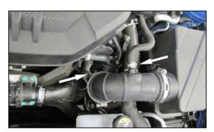
3. Release the spring clamps that secure the two vent lines attached to the driver's side intake tube, then remove the vent lines from the intake tube.
