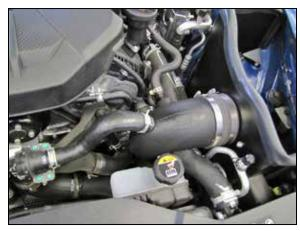
13. Install the provided filter adapter into the heat shield so that it goes through the heat shield and into the coupler on the intake tube. Secure the adapter to the heat shield using the provided hardware and then adjust the intake tube and couplers for best fit and secure with the provided hose clamps. Connect the vent lines to the fittings in the intake tube and install the factory passenger BOV hose and secure with the factory clamps.
