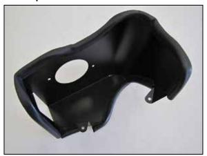
11. Trim and install the edge trim 35", 16" and 2-1/2" onto the driver's side heat shield (20-8633) as shown.
