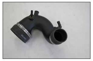
10. Install the provided couplers (5-222N & 08761) onto the Drivers side intake tube (9-0459) and then install the 90° and straight vent fittings as shown. NOTE: NPT fittings are easy to cross thread. Install the vent fitting "hand" tight, then turn it two complete turns with a wrench.
