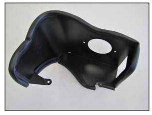
14. Trim and install the edge trim 35", 16" and 2-1/2" onto the passenger side heat shield (20-8634) as shown.
