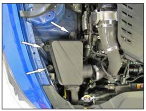
8. Remove the three bolts that secure the passenger side air filter housing to the inner fender, loosen the hose clamp that secures the intake tube to the air filter housing and disconnect the tube. Remove the passenger side air housing from the vehicle.
