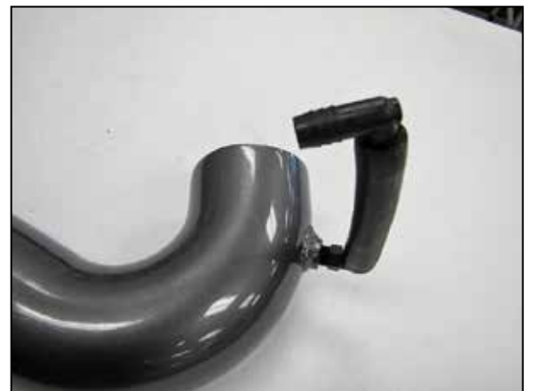
17. Install the provided crank case vent and 90° union fitting onto the AEM® intake tube as shown.
