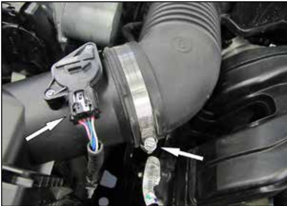
6. Loosen the hose clamp that secures the intake tube to the air filter housing and disconnect the mass air sensor electrical connection.
