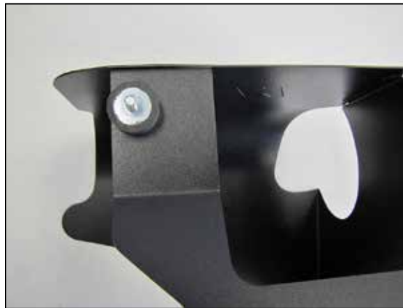
11. Install the rubber mounted stud onto the heat shield as shown.
