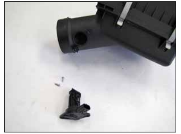
14. Remove the mass air sensor from the factory air filter housing.
