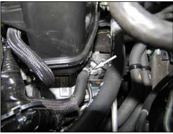
4. Release the spring clamp and then disconnect the crank case vent from the intake plenum.
