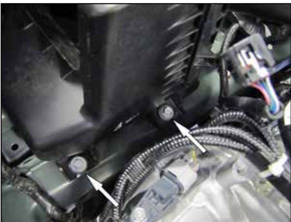
8. Remove the two bolts that secure the factory air filter housing to the frame rail.
