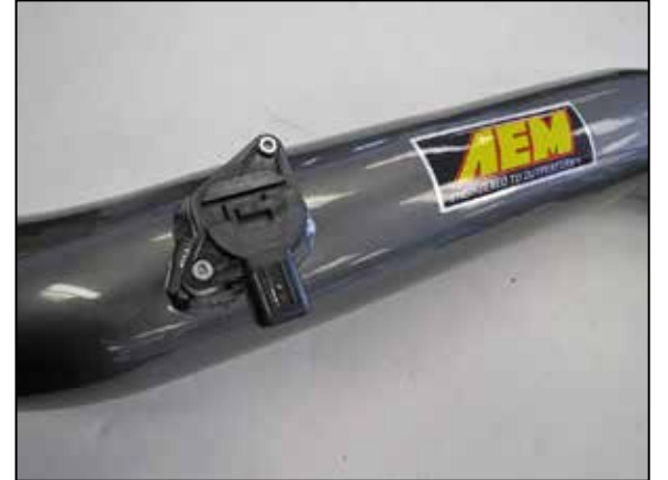
15. Install the mass air sensor into the AEM® intake tube and secure with the provided hardware.
