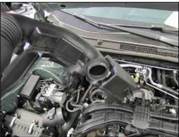
7. Remove the factory intake tube from vehicle.
