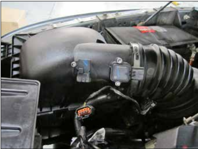
a. Unplug the factory MAF and IAT Sensor connectors.
