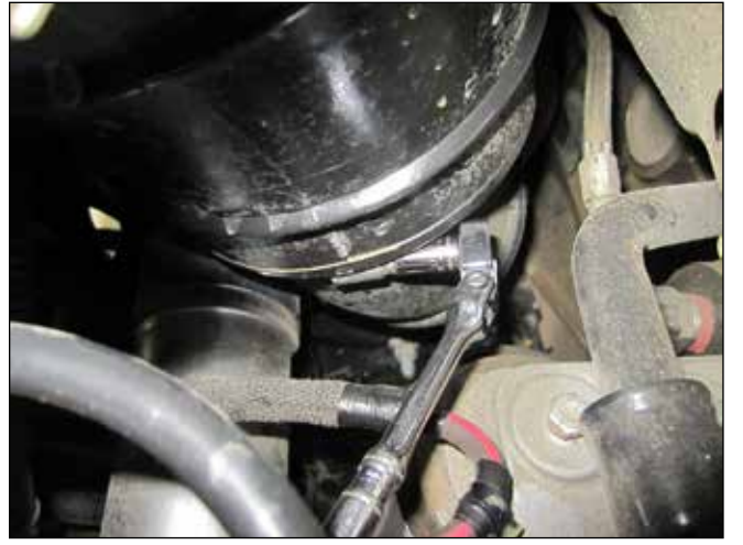
d. Loosen the hose clamp securing the factory inlet hose to the turbocharger.
