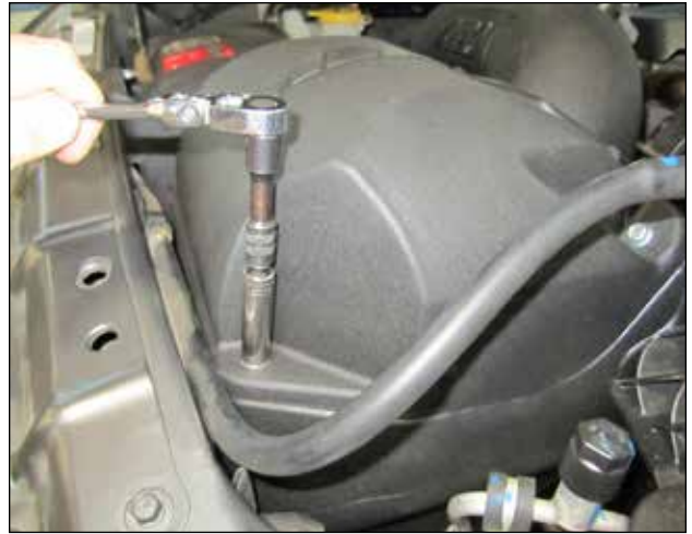
u. Install and tighten the four 6mm bolts(1-2038) for the air box lid.
