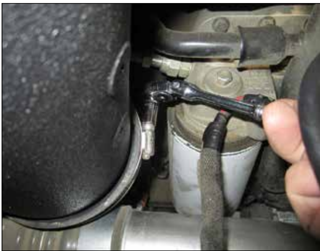
v. Adjust the intake tube for maximum clearance and tighten the hose clamp on the turbo coupler to the AEM intake tube.
