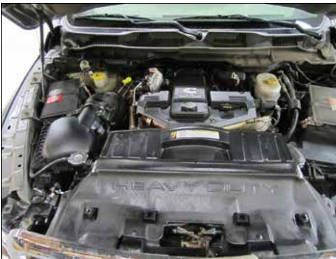
Stock Intake system installed
