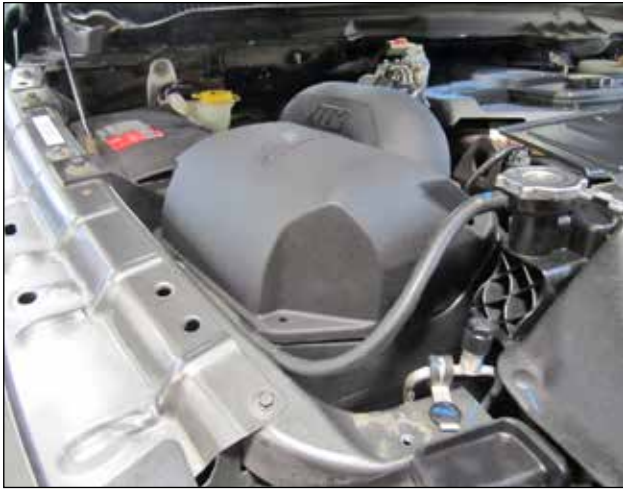
t. Set air box top(9-0404) in place.
