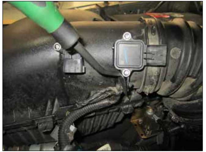
b. Pull out the wire harness clip on the air box for the connectors.
