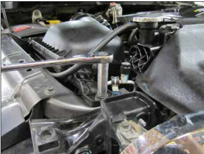
c. Remove the 13mm bolt securing the air box base to the radiator support.
