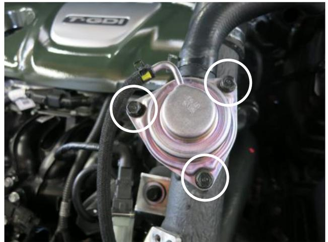
d. Remove the 3 bolts securing the recirculation valve to the stock intercooler pipe, then move the valve to the side of the engine compartment. Note: bolts and O-ring will be reused in step 3n.
