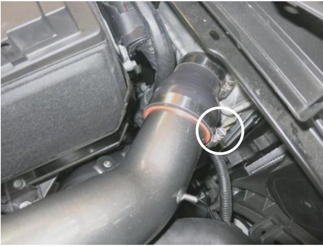
k. Tighten hose clamp circled at the intercooler to 30 in-lbs
