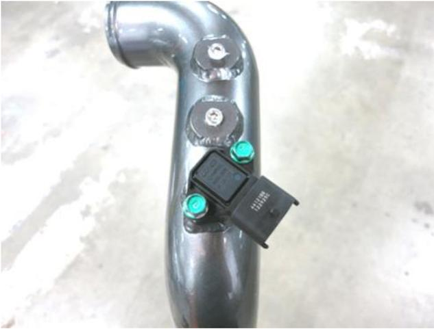
a. Install the 2 NPT plugs into the AEM intercooler pipe with Teflon tape or pipe sealant. Then, install the pressure sensor with M6 bolts removed in step 2n.
