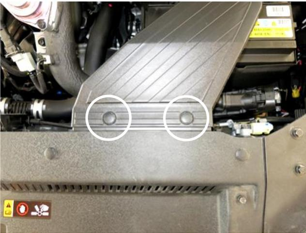
a. Remove the two clips securing the stock air scoop and remove the scoop from the vehicle.
