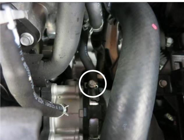
i. Loosen the hose clamp at the throttle body. Note: A hose clamp cap that covers the slot may be present. You can pry it off with a screwdriver or pliers.
