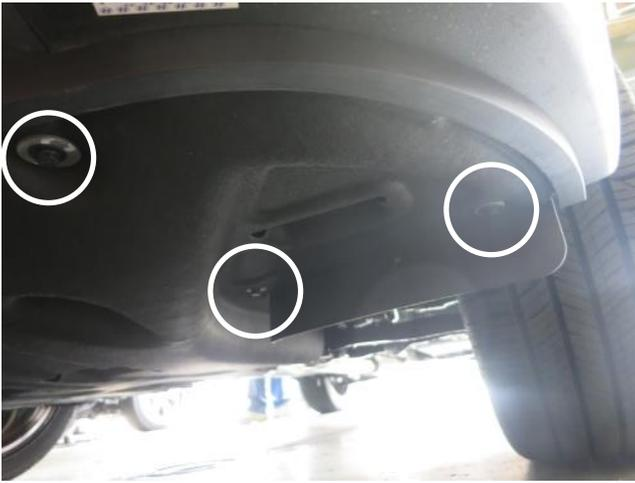
k. Remove the 17 bolts that secure the splash shield to the vehicle. Note: The small oil access cover does not need to be removed from the shield and not all of the bolts are pictured above.
