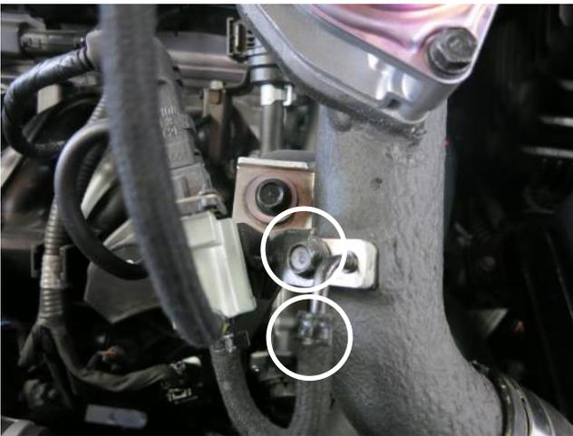
c. Remove the M6 bolt securing the electrical connector. Release the tension on the spring clamp and remove the vacuum hose from the nipple. These will be reused in step 3l & 3m.
