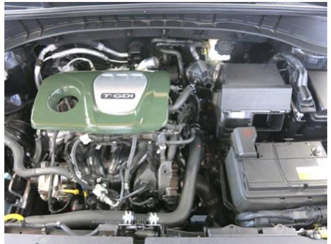
h. Remove the upper intercooler pipe from the engine by taking it off from the turbo compressor first, then from the intercooler inlet.
