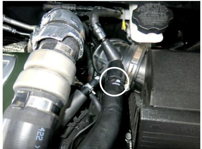
b. Squeeze the spring clamp and work the clamp back off of the turbo recirculation valve hose. Disconnect the hose from the stock intake tube.
