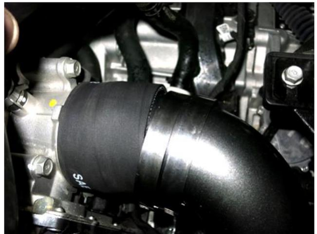
d. Install the provided coupler onto the throttle body and install the AEM lower intercooler pipe into the coupler along with hose clamps. Note: Warm soapy water will help with installation.
