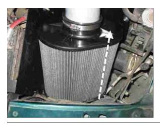
f. Reinstall filter onto vehicle.
