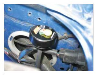
d. Attach one end of 5/32" hose to elbow on filter, and the other end to the filter minder nipple. Trim excess hose.
