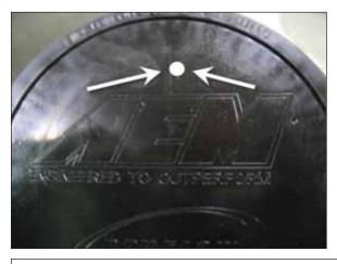
b. Drill 1/8" hole in lid of filter. Make sure no debris from the drilling operation gets inside the filter.
