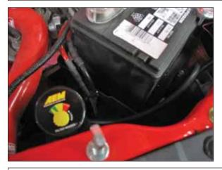
c. Mount under hood in a suitable location using the enclosed bolts and nuts. Alternatively, you may also use zip ties or another method to securely attach the filter minder remote mount assembly to the vehicle. See images for step 3c and 3d as examples for mounting the filter minder
