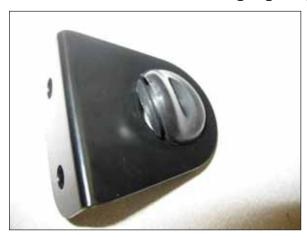
a. Install 3/4" grommet in remote mount bracket.
