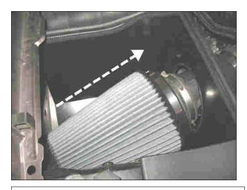
e. Reinstall the air filter onto vehicle. Proceed to step 3.
