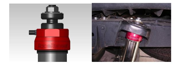
Using the stock lower nuts and bolts, install the lower end of the shock to the stock mounts. Torque the nuts to 75 ft-lb.
