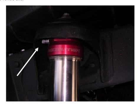
9. Place the second bushing on the stud, on the top side of the frame, followed by the washer and the locknut. Hand-tighten the locknut, until the nylon engages and the nut starts to tighten.
