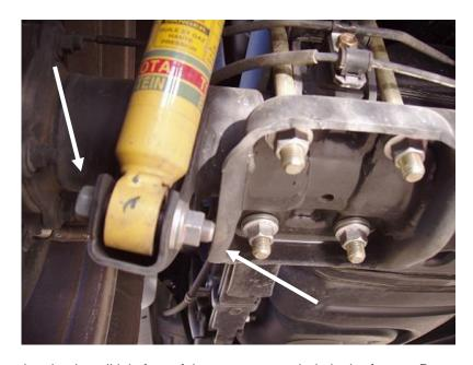
7. Lower the shock until it is free of the upper mount hole in the frame. Remove the shock.
