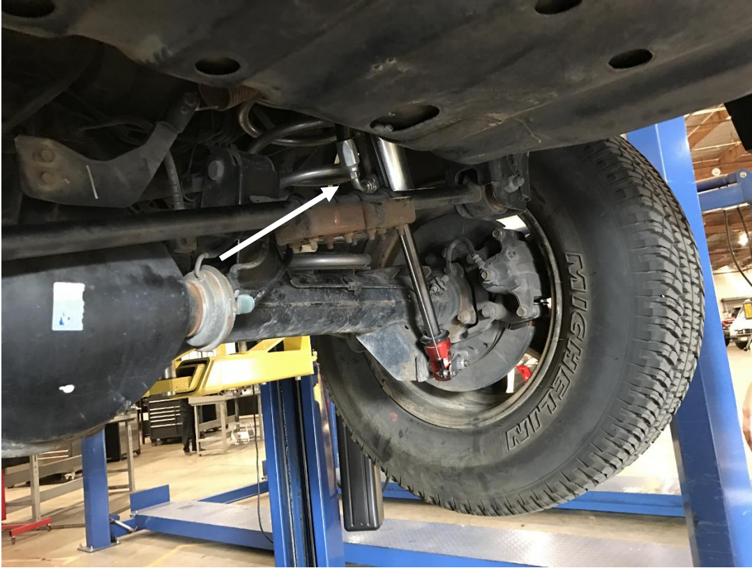
LEFT side shock with LONGER hose pointing to the left:
