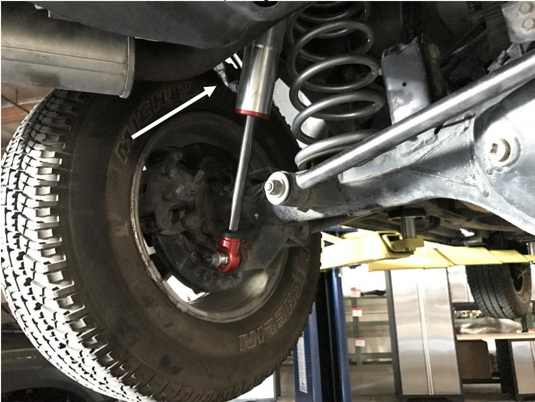
LEFT side shock with LONGER hose pointing to the left:
