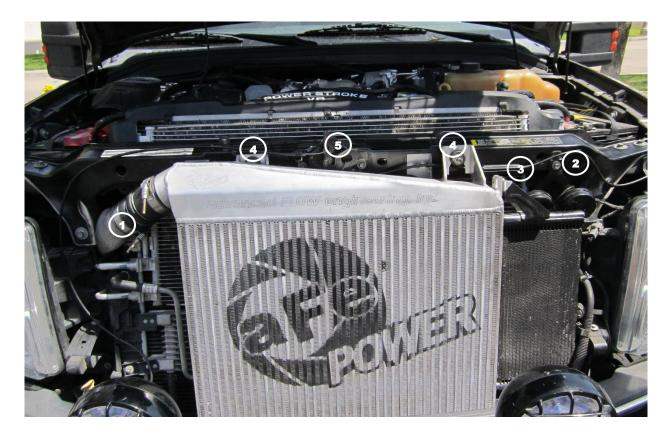
Note: It is recommended to trim the core support for the fitment of this charge pipe.
