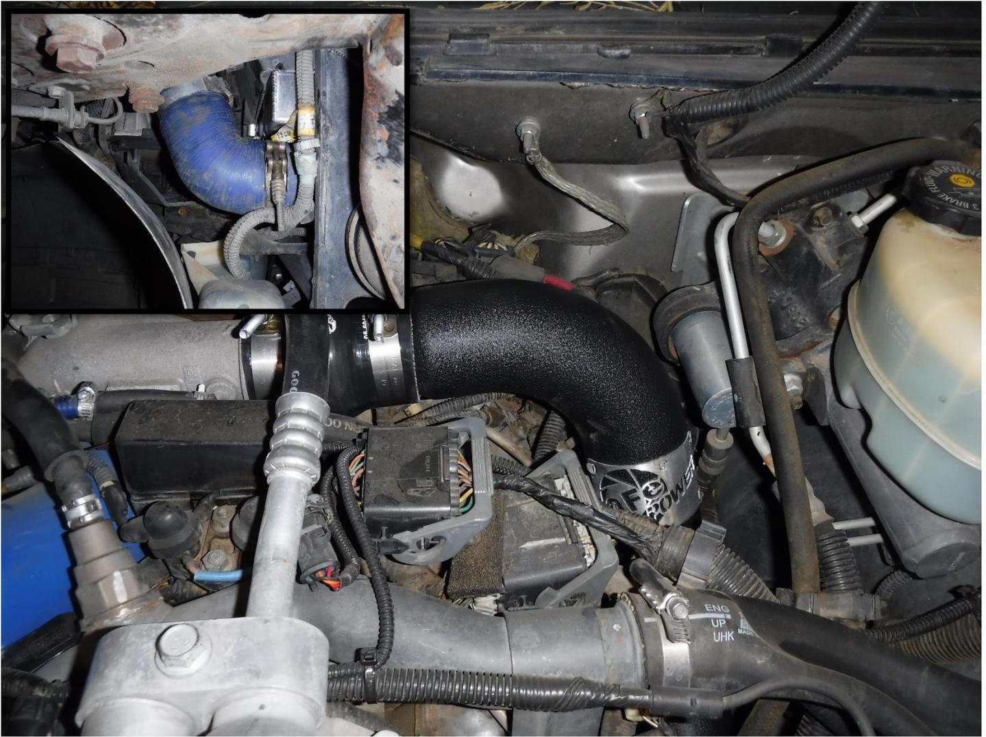
53. Reinstall the hot side intercooler tube into the vehicle.
