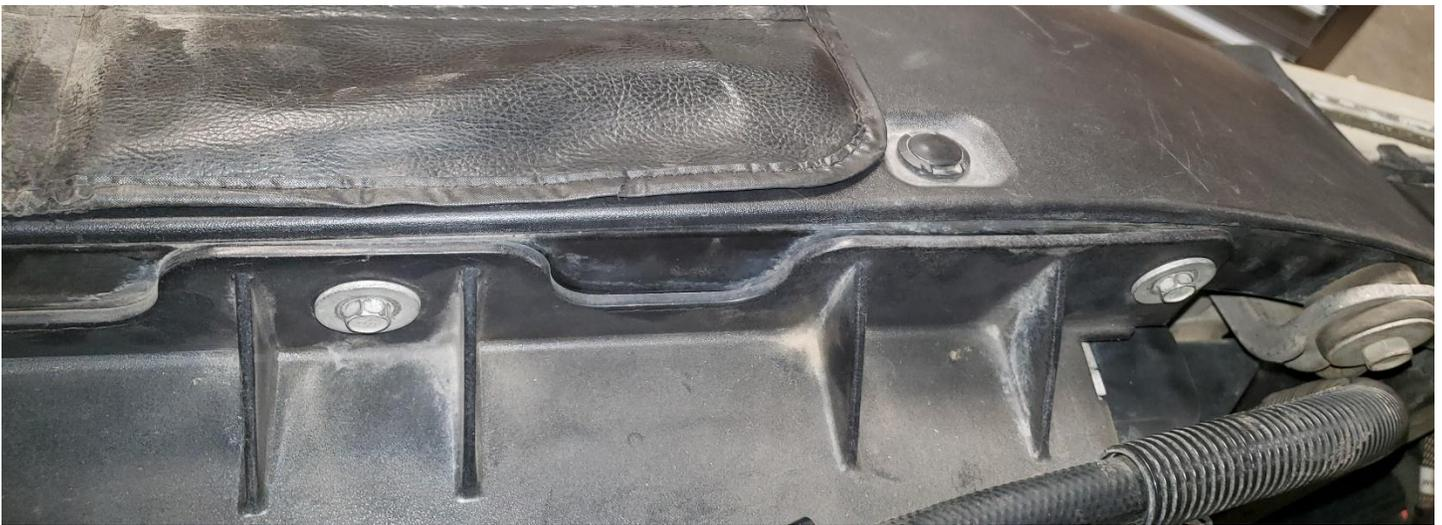
23. Unclip the A/C hose from the upper fan shroud.
