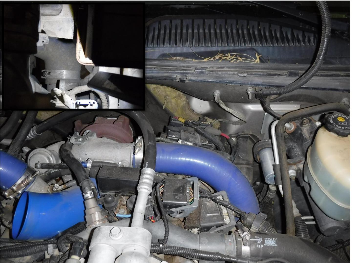
18. Loosen the clamp securing the hot side intercooler tube coupling to the turbo.
