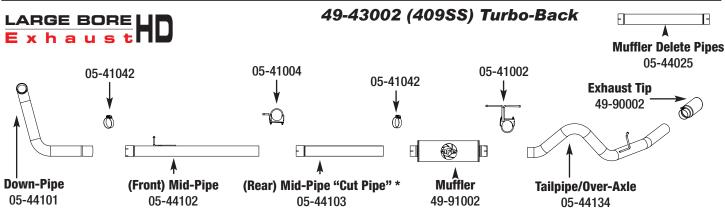
1: (Read Instructions prior to installation) Remove your stock exhaust from the rear of your truck working your way forward. Take caution not to damage the factory isolation mounts. If you want to remove the OE downpipe in one piece or without cutting, you must remove the transmission cross member and disconnect the dip-stick tube & sway bar end links. It is recommended to not fully tighten the clamps until the entire system has been installed.
