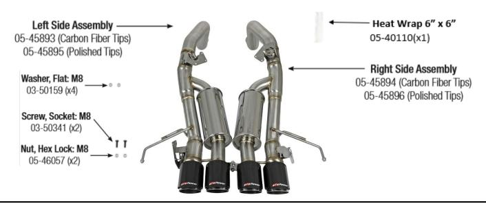
aFe POWER recommends professional installation on this product. Thoroughly inspect the aFe POWER exhaust system to make sure there is no damage from shipping (if damage is noted, immediately contact aFe POWER customer service). Allow time for your vehicle to cool down prior to installation. When working on your vehicle proceed with caution. Wear protective safety equipment; eye goggles and gloves to ensure a safe installation.
