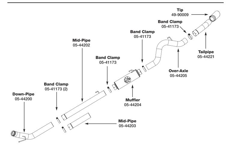
**Step 1:** (Read Instructions prior to installation) Remove your stock exhaust from the rear of your truck working your way forward. It may be necessary to cut the pipes if the slip joints are stuck. Take caution not to damage the factory isolation mounts as they will be reused. **It is recommended to not fully tighten the clamps until the entire system has been installed.**
