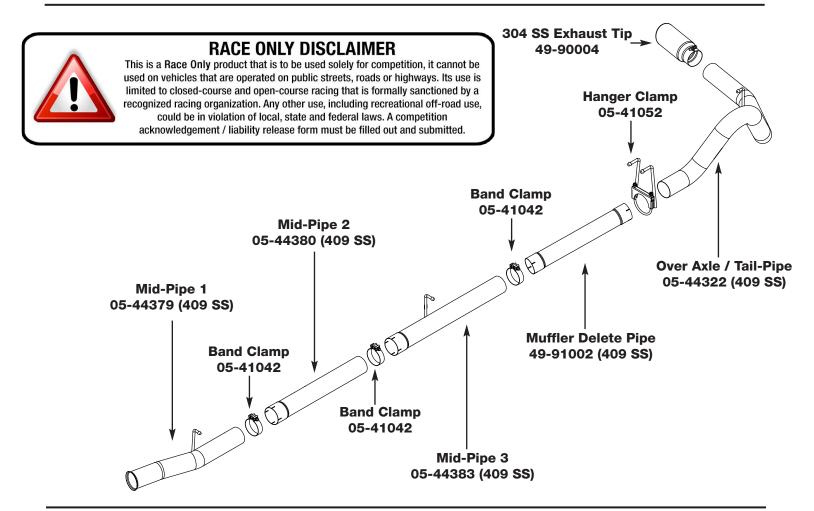
**Step 1:** (Read Instructions prior to installation) Remove your stock exhaust from the rear of your truck working your way forward. It may be necessary to remove front crossmember for turbo down pipe removal. Take caution not to damage the factory isolation mount as they will be reused. Disconnect sensors at the connections. Take caution as not to damage any sensors. It is recommended to not fully tighten the clamps until the entire system has been installed.
