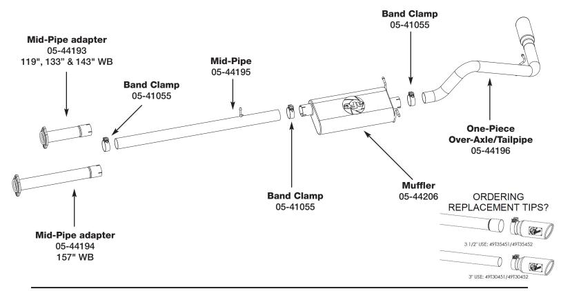
**Step 1:** (Read Instructions prior to installation) Remove your stock exhaust up to the catalytic converter from the rear of your truck working your way forward. Take caution not to damage the factory isolation mounts as they will be reused.
