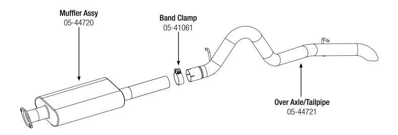
**Step 1: (Read Instructions prior to installation)** Remove your stock exhaust from the rear of your truck working your way forward. Take caution not to damage the factory isolation mounts as they will be reused. It may be helpful to lubricate the isolation mounts prior to disassembly. It is recommended to not fully tighten the clamps until the entire system has been installed.
