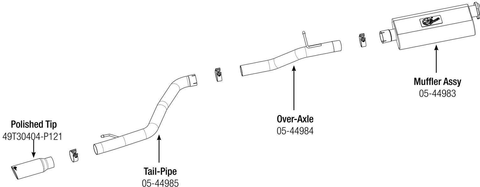
Professional installation is highly recommended. (Read instructions prior to installation) This system requires an aftermarket electronic module To, work properly with the vehicle. **Make sure to always have at least (2) stands or jacks on hand to support the removal of OE system. As, well as for the installation of aFe system. Any Removal of rubber isolation mounts may require using a spray lubricant such as WD40 and a pry bar.**
