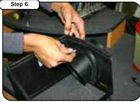
Step 6 Place the intake tube into the housing and secure with the provided nuts, bolts, and washers. Place the trim seal along the edge of the housing.
