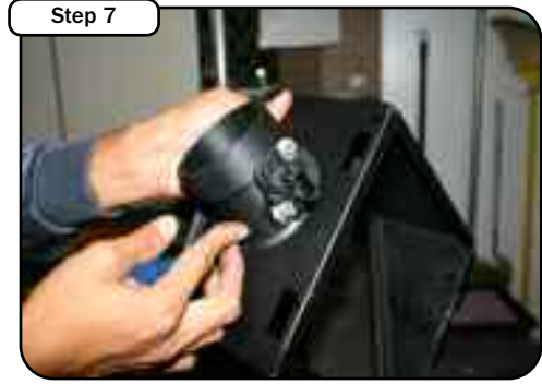
Step 7 Transfer the MAF sensor to the intake tube. Use the supplied gasket, nylon spacers, and screws. Pay close attention to the flow of the MAF sensor when inserting the sensor into the tube.
