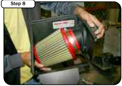
Step 8 Insert the new air filter into the intake tube. Install the filter from the bottom of the housing for ease of installation.
