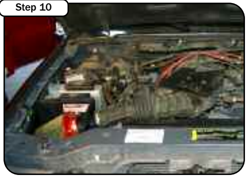
Step 10 Place enclosed CARB EO sticker on or near the device on a smooth, clean surface. EO identification label is required to pass the smog inspection. Your installation is now complete. Make sure all hoses and clamps are tight and that all electrical components are secure. Check and retighten connections and filter after a few hours of operation. Close hood slowly to verify hood clearance.
