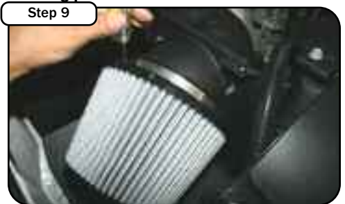
Carefully install the 6" aFe air filter and tighten with 5/16 nut driver.
