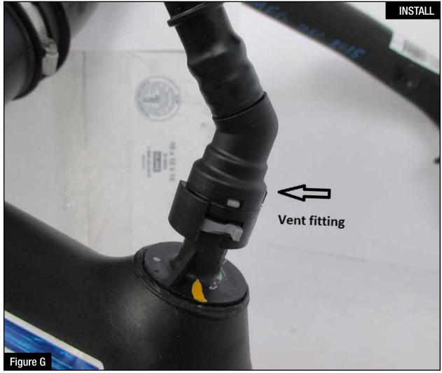
Refer to Figure G for Step 16 (For V6-3.5L (tt) only, not necessary on V6-2.7L (tt) ) Step 16: Locate the valve cover vent tube that feeds into driver's side turbo inlet. It is not necessary to remove the engine cover.
