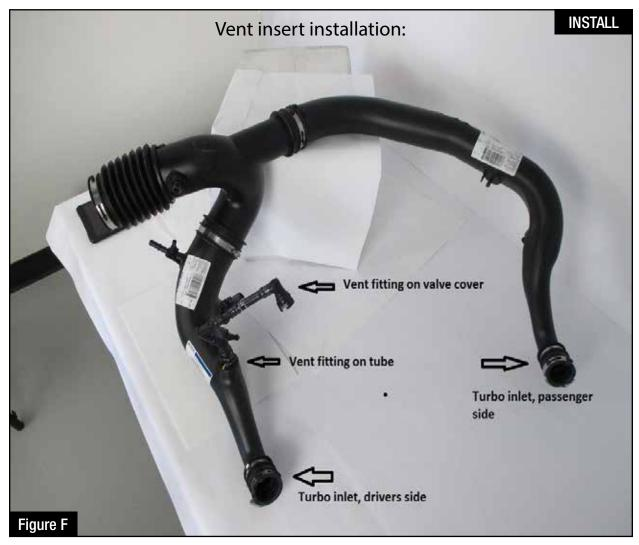
Refer to Figure F for Step 15 (For V6-3.5L (tt) only, not necessary on V6-2.7L (tt) )
