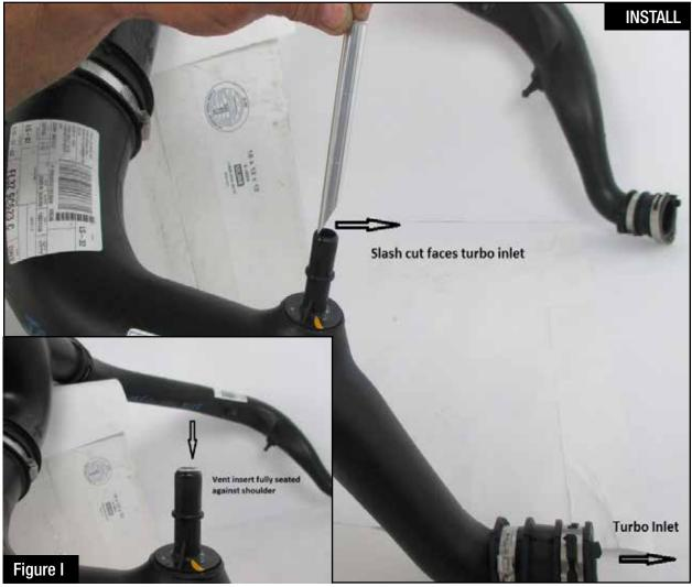
Refer to Figure I for Step 18 (For V6-3.5L (tt) only, not necessary on V6-2.7L (tt)) Step 18: Insert vent fitting with slash cut facing turbo inlet. It should not be a loose fit. It is direction dependent and must not rotate once installed.
