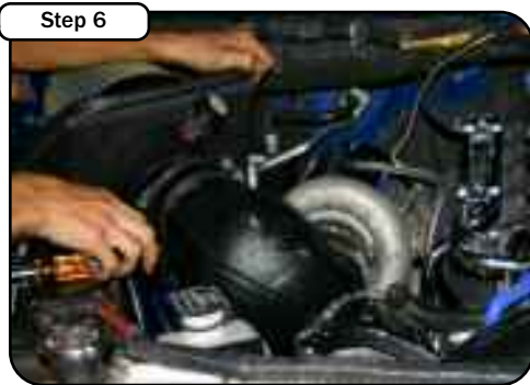
Tighten all the clamps snug but do not overtighten.
