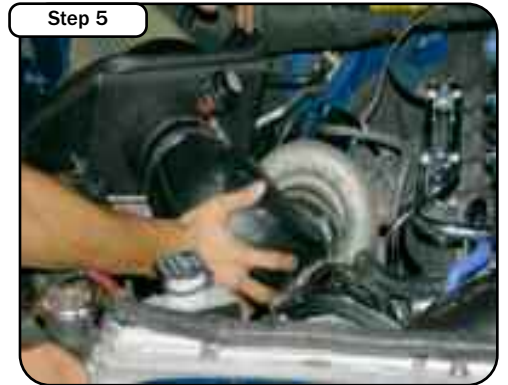
Position the assembly into the intake kit and tighten clamps.
