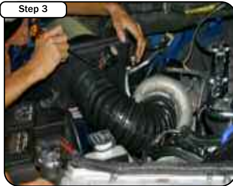
Loosen the two hose clamps on the intake duct. Remove intake duct out of the engine bay.
