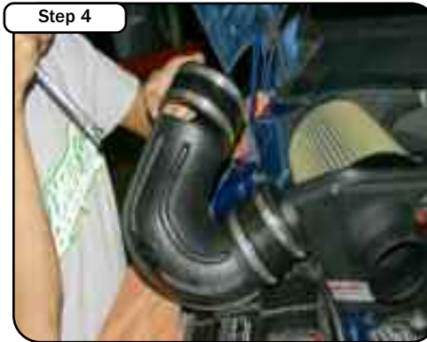
Place the couplers and clamps on the intake tube. Do not tighten clamps at this time.
