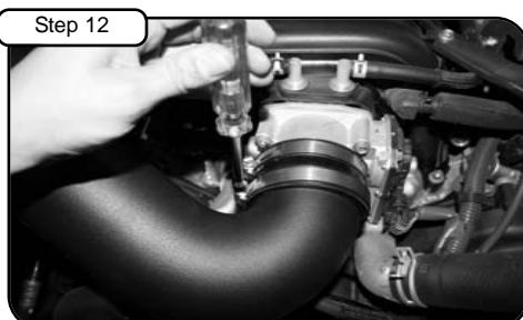
Tighten clamps at throttle body with 5/16" nut driver.
