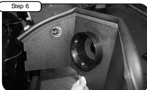
Install filter adaptor to inside of housing using 5 button head screws and wavy washers. Tighten using 5/32 hex key. Install 3/4" trim seal to housing.
