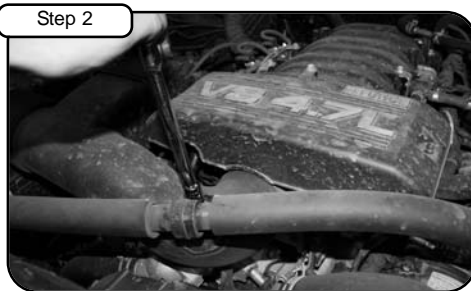
With 10mm wrench or socket, loosen bolts on engine cover. Loosen bracket holding AC line to tube and remove. Disconnect MAF sensor harness.
