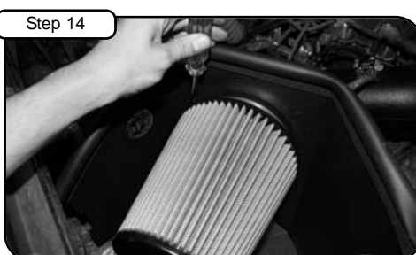
Install air filter and tighten using 5/16" nut driver. Re-install engine cover.
