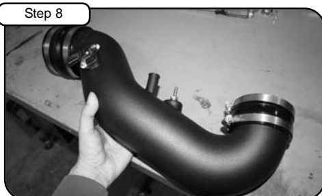
Remove MAF sensor from stock air box. Install into new tube using gasket, 1/8" nylon spacers, and M4 screws provided. Install brass nipple to tube and tighten. Install couplers with clamps on tube.
