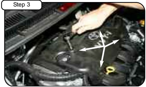
Remove engine cover with 10mm socket.
