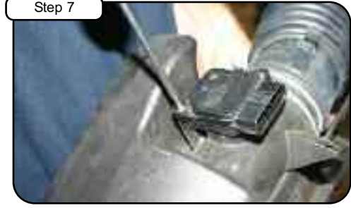
With phillips screwdriver, remove MAF sensor. Install both 7/16" trim seal to new aFe housing. (as shown in step 8)
