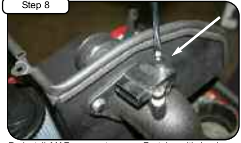
Re-install MAF sensor to new aFe tube with hardware provided (make sure gasket and nylon spacers are between tube and sensor) using flat head screwdriver. Install tube to outside of housing and tighten using M6 screw, wavy & flat washer with M6 nut and tighten.
