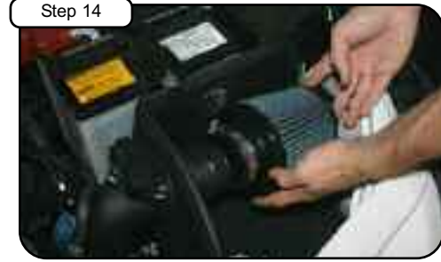
Re-connect MAF sensor. Place high FLOW filter into housing and tighten using 5/16" nut driver.
