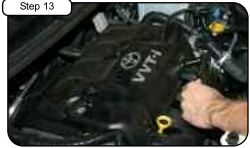
Install engine cover and use the 4 cover nuts from step 3 and tighten using 10mm socket.
