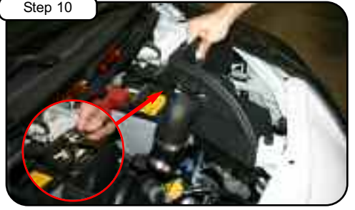
Install 2-1/4" elbow with clamps provided to intake tube. Now install intake system into vehicle. Re-install 10mm nut on battery bracket and tighten.
