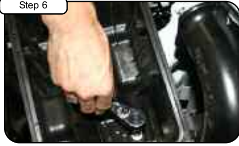
With 10mm socket, loosen the 2 bolts that hold in bottom half of stock air box and remove.
