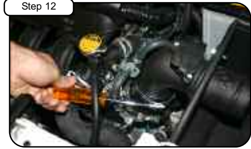
Attach other side of crank case line to 1/2" hose fitting with mini clamp and tighten. With 5/16" nut driver tighten clamps at elbow coupler.
