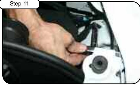
Using M6 nut and wavy washer provided tighten front of housing to headlight assembly using 10mm socket.
