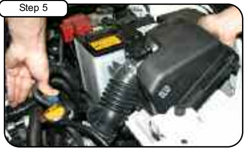
Loosen intake clamp with 10mm socket and un-clip the upper half of stock air box. Remove OE intake out of vehicle.
