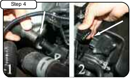
1) Remove the crank case line from engine and stock intake. 2) Disconnect MAF sensor.
