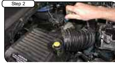
Use 5/16" nut driver to loosen clamps on OE tube at turbo/air box and remove.
