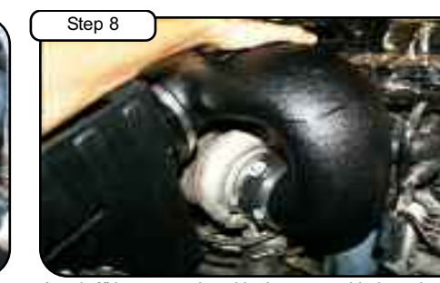
Attach 6" hump coupler with clamps provided to tube and install tube to turbo and filter adaptor. Adjust and tighten all clamps with 5/16" nut driver.
