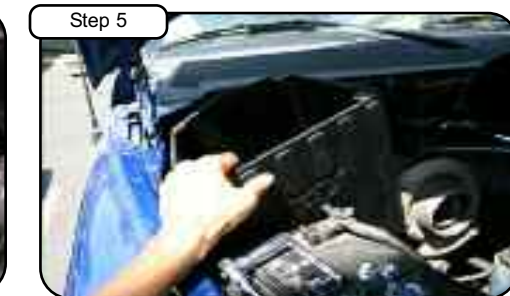
Install housing into vehicle and position. Press down firmly to seat. If this is installed on a 4x4 model, a clearance hole will need to be drilled for the upper shock stud.
