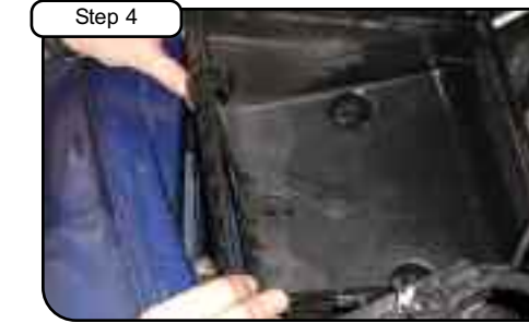
Carefully lift and pull bottom half of air box to remove from vehicle. Transfer rubber mounts to the new housing.
