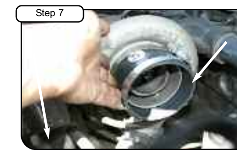
Install high temp coupler to turbo using clamps provided. Do not tighten.
