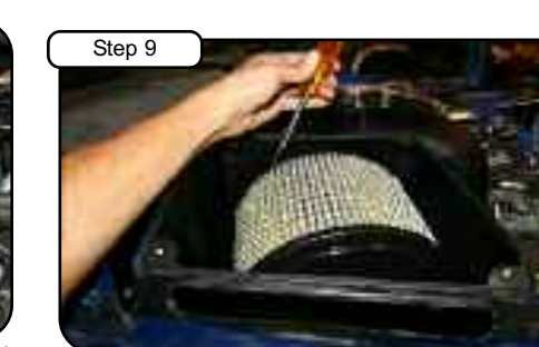
Install air filter and tighten with 5/16" nut driver.
