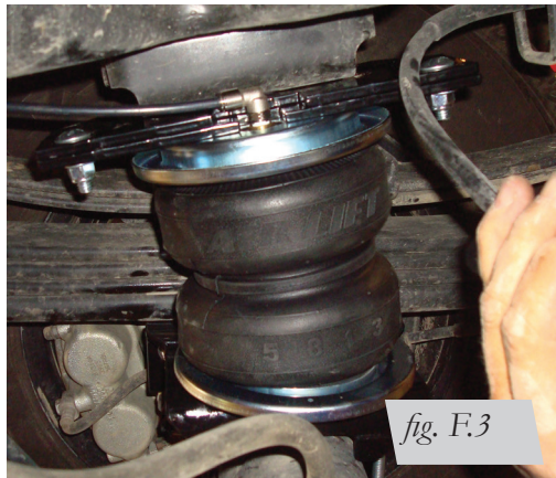
Inside view of the driver's (left) side installation.
