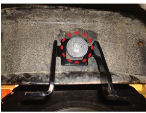
Passenger's (right) side upper brace shown with hardware supplied in place.
