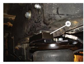
The spacer (H) must be parallel to both the frame and upper bracket. Raise axle or lower frame until the spacer touches the frame on both sides.
