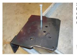
3/8-16 X 7" carriage bolts go into the square holes. Passenger's (right) side shown.
