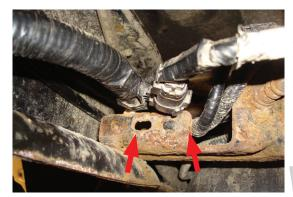
Remove the line holders from the gas/DEF tank bracket for easier access to the upper brace hardware.
