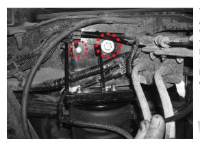
Tighten the M8 and 1/2" (or 3/4" from the existing fifth-wheel hitch) hardware securely. Repeat for the hardware on the opposite side.
