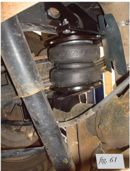
Passenger's (right) side view of the kit installed from forward of the axle.
