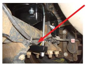
It may be necessary on some models to not tighten the axle clamp bar evenly on the passenger's (right) side so that the clamp bar will clear the hard brake line.
