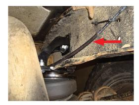
Air line thermal sleeve shown in place on the right side (passenger) of the vehicle. Make sure thermal sleeve is pushed up against the fitting once the air line is installed.
