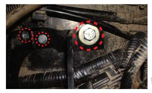
Driver's side brace shown with supplied hardware in place. Existing fifth-wheel hardware which may have been removed may look different.
