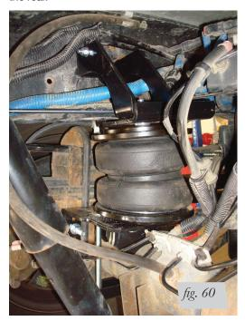
Driver's (left) side view of the kit installed from rear center of vehicle.
