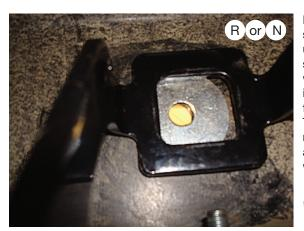
For the passenger's (right) side, before inserting the upper brace hardware, make sure that the 1/2" thick washer (R) or (N) is installed in between the brace and frame (see Step 2). Note: The 1/2" thick washer (R) is not a half inch thick. It has a 1/2" hole and is a thick washer.
