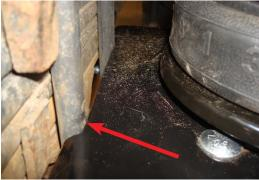
Bracket must be up against the stock U-bolts and the flanges of the lower bracket must be locked forward and behind the stock U-bolts.
