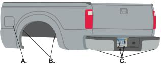
\* For LoadLifter 5000 Ultimate Plus kits, the recommended location for the Schrader valves is the rear bumper area or license plate.
