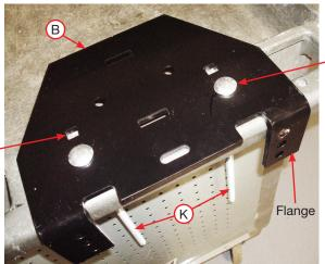
For models with sway bars, right (passenger side) only, use these holes for installing Carriage Bolts (B).
