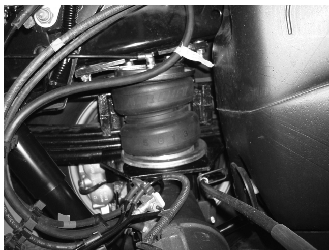
Inside, over axle view of passenger's (right) side installation.
