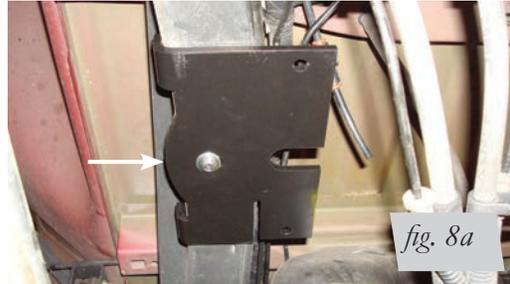
LH (driver) side. Push bracket against frame and torque to 38 lb.-ft (52Nm).
