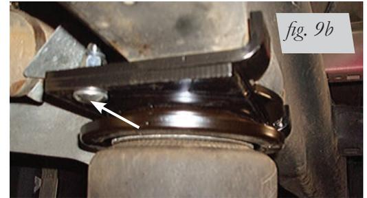
Right hand assembly (passenger side) attached with carriage bolts (R), flat washers (M) and nylon lock nuts (U). Torque to 31 lb.-ft (42Nm).
