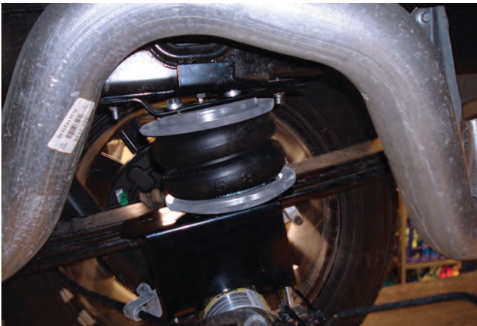
Inside view of right-side mounted assembly
