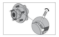
**NOTICE**: Make sure the surface and splines on original hub and axle are clean and free of all dirt and debris, a brake parts type cleaner may be needed. Splines should be free of burrs and any imperfections that could interfer with the installation and proper function of new hubs. A small amount of SAE 30 type weight oil is recommended as a lubricant on all spline surfaces to aid in the installation processs and to help with proper function of new hub.
