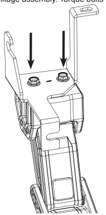
Locate mounting points on rearmost body mount on **Passenger side** of vehicle. Using a 15mm deep socket to remove conical washer nut. Next use 21mm socket to back out bolt at frame. **Only remove enough to slide bracket into position.**
