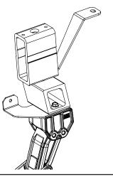
Slide threaded plate into bed channel and line up threaded locations to pre drilled holes.
