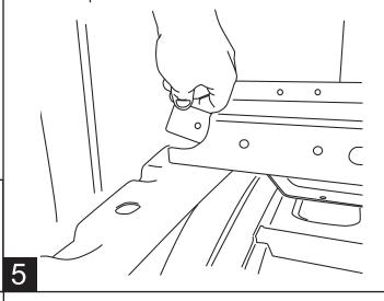
Using an 18mm Socket assemble Frame mount bracket to bed mount bolt. Do not tighten bolts
